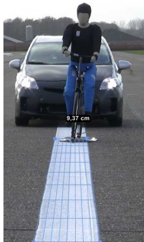
Figure 2-7: Example of computation of lateral accuracy at impact point using video analysis in the longitudinal scenario
