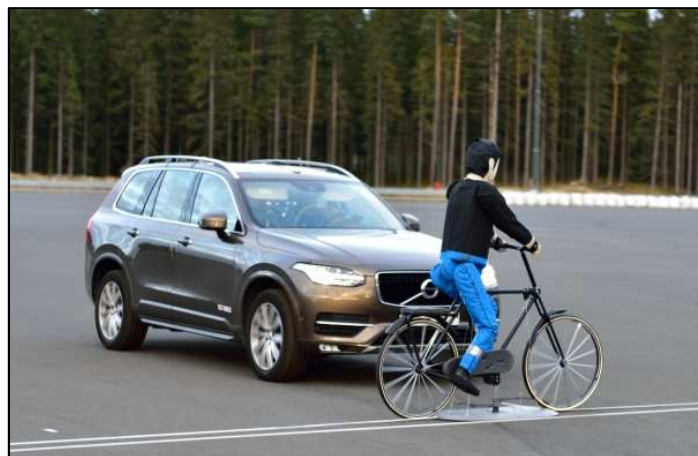
Figure 2-5: Example of the test setup: XC90 in near side crossing test (CVNBU)
