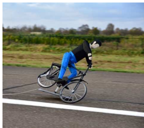
Figure 3-9: Dummy target right after the moment of impact with a 60km/h tests. Dummy did not release from platform and damage is visible to rear wheel. However, testing could continue within minutes.
