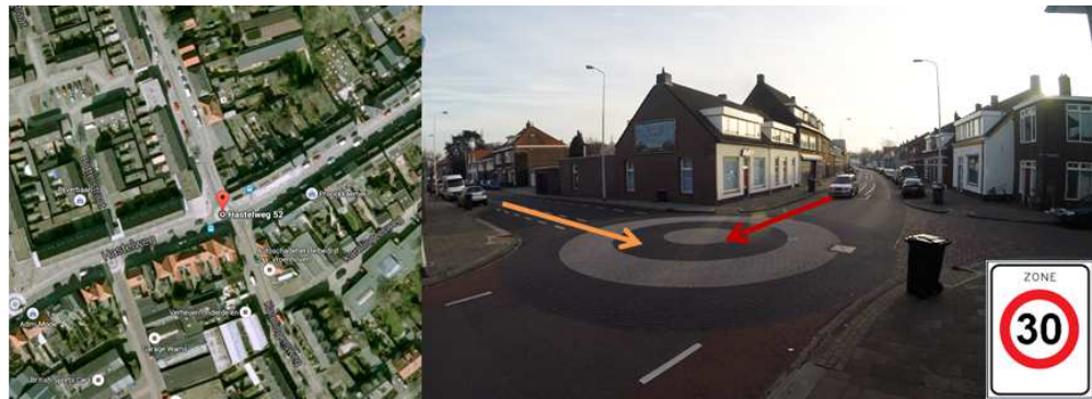
Figure 8 Top view and camera overview of selected crossing in Eindhoven. Cyclists (orange arrow) approach the cars (red arrow) from the right, where the cyclists have right of way. Speed limit of the cars in this area is 30 km/h. The garbage bin containing the measurement equipment can be seen at the right side of the figure.
