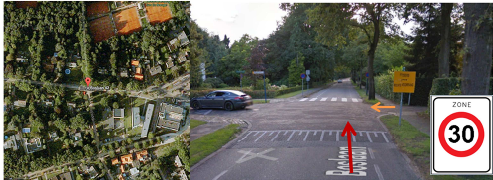
Figure 7 Top view and car view of selected crossing in Son en Breugel. Cyclists (orange arrow) approach the cars (red arrow) from the right, where the cyclists have right of way. Speed limit of the cars in this area is 30 km/h. The yellow sign at the right was not present during the measurement day.
