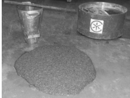
Figure 3: Example of workability for PU/PFA showing slump flow after 4 min.
