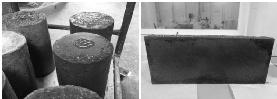
Figure 7: (Left) Recipe 1 after 420 freeze-thaw cycles. (Right) Recipe 2 panels. [Chozas et al. , 2015]
