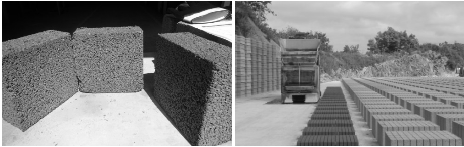
Figure 8: Replication of building blocks. (Left) Laboratory production. (Right) Factory trials
