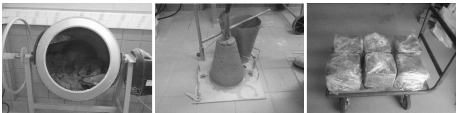
Figure 9: Concrete mixer (Left), Slump measurement (Centre) Cubic moulds covered for curing (Right)
