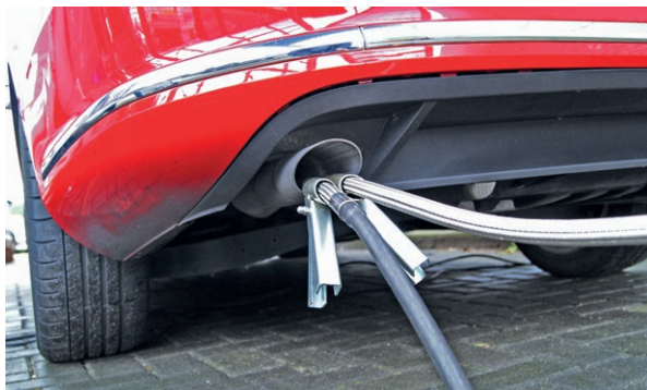
Figure 13. The PM emissions from diesel vehicles can be determined during the APK using a smoke meter. For late model diesel vehicles, however, it is permitted to simply check the OBD system for fault codes (photo: TNO).
