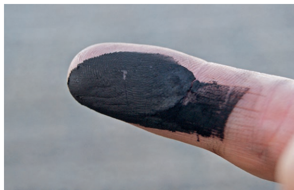
Figure 3. Black deposit on a finger after wiping deposits from a diesel exhaust pipe. The black emission produced when burning diesel is popularly referred to as 'soot.' Soot, however, is not a scientific term. A particulate filter captures all solid particles created during the combustion of diesel. Most of it is elemental carbon, referred to as EC (photo: TNO).
