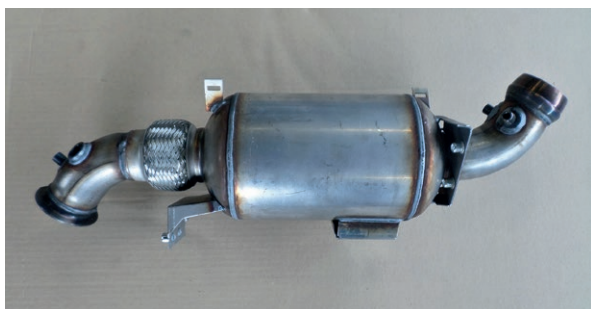
Figure 1. A particulate filter for a passenger car, as part of the exhaust system. The filter element (see figure 2) is located in the metal canister (photo: Topcats).
