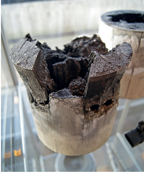
Figure 7. An irreparably damaged diesel particulate filter. Continuing to drive with a restricted particulate filter can cause irreparable damage to the DPF and even serious engine damage (photo: TNO at Digicar Engineering).
