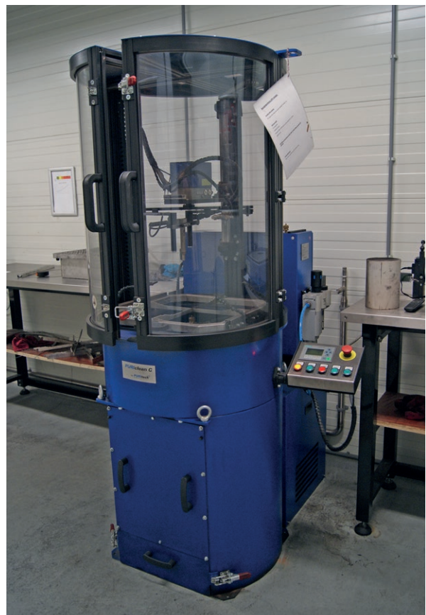
Figure 8. A kiln cleaning involves placing a DPF in a kiln for several hours (above). After removal from the kiln the ash is blown out of the filter (bottom) (photo: TNO at Digicar Engineering).
