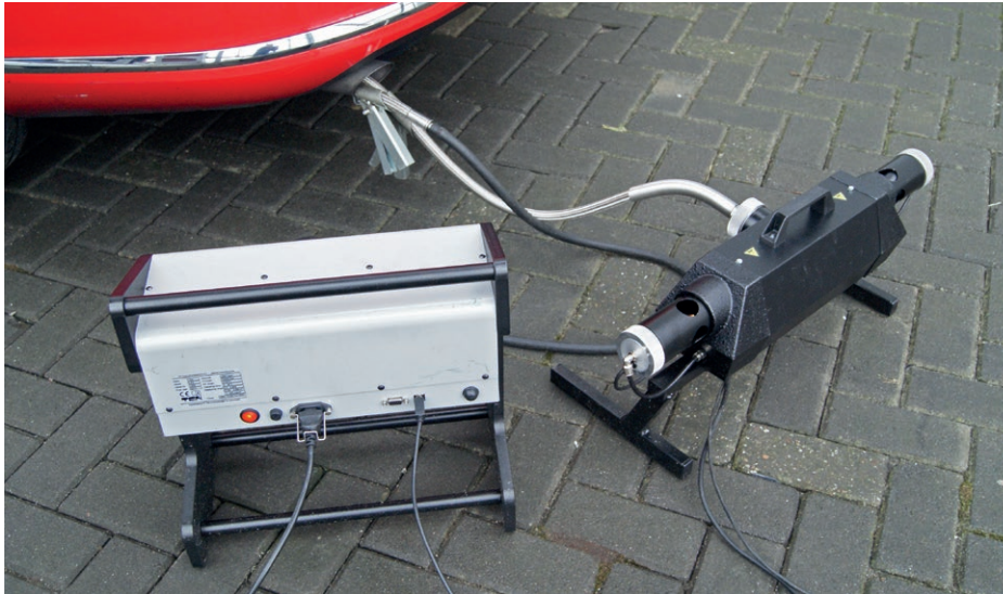
Figure 14. In the 2016 study, the absorption coefficient values were measured with two types of smoke meter: a conventional or 'standard' smoke meter (or opacimeter) as is currently used for the APK (right), and a state-of-the-art, 'improved' smoke meter (or opacimeter) (left) with greater sensitivity than the old meters. A smoke measurement is carried out 'at free acceleration': the maximum smoke emission is measured while the throttle pedal is depressed fully (photo: TNO).
