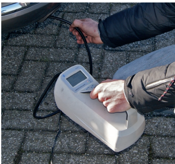
Figure 15. In addition to the conventional smoke measurement, the number of particles (Particle Number or PN) in the exhaust gases of the 213 diesel vehicles was measured using a particle counter. The sampling hose is placed in the exhaust tailpipe while the warm engine runs at idle (left). The device displays the number of particles per cm 3 ('10' in the photo at the right) (photo: TNO).
