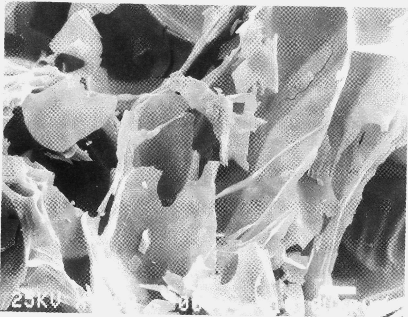
Figure 4.2. SEM of the internal pores of perlite; critical point dried, bar = 10 \mu\text{m} .
