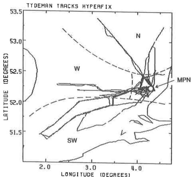
Figure 1: Composite sailing schedule of Hr.Ms. Tydeman. The position of the MPN tower is indicated by the arrow. The dashed lines define the regions used in the assessment of spatial variability of the aerosol extinction.
