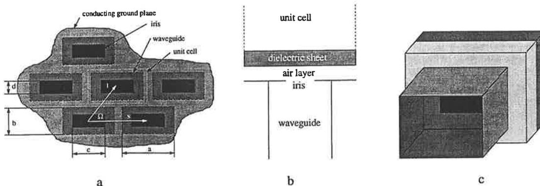
Figure 1: Waveguide phased array antenna unit cell
