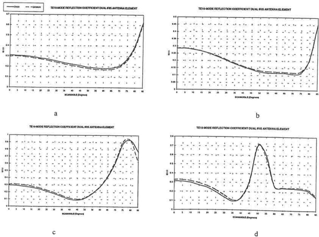
Figure 10: Active element reflection coefficient vs. scan angle for different frequencies
