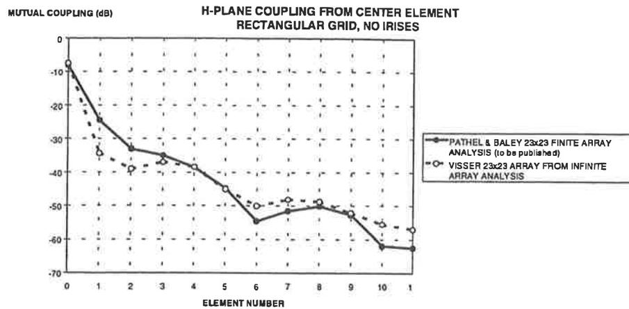
Figure 2: Code-to-code validation finite waveguide phased array antenna
