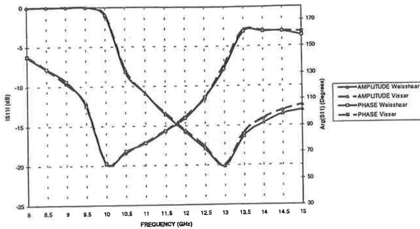
Figure 7: Reflection coefficient H-plane step discontinuity
