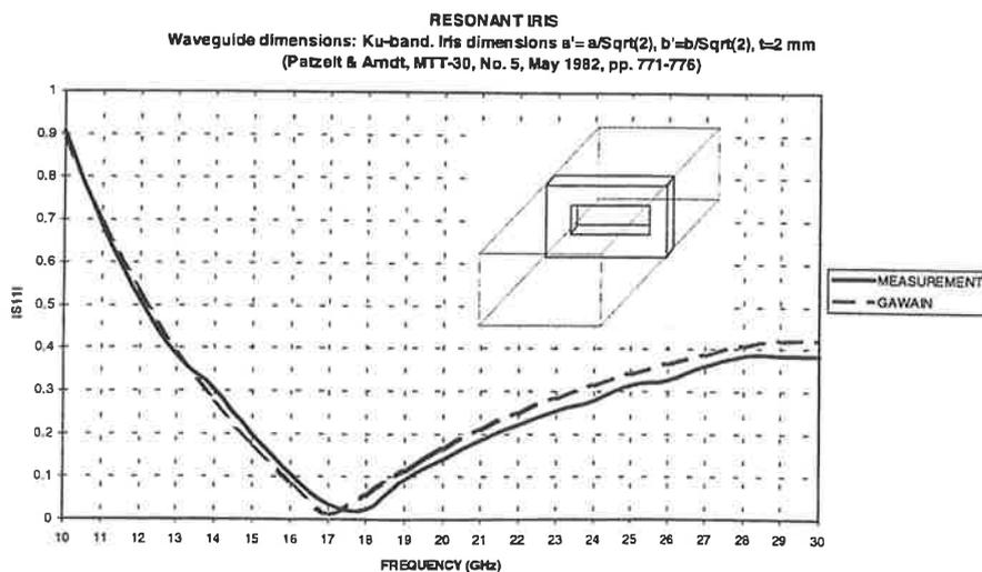
Figure 6: Reflection coefficient resonant iris of finite width
