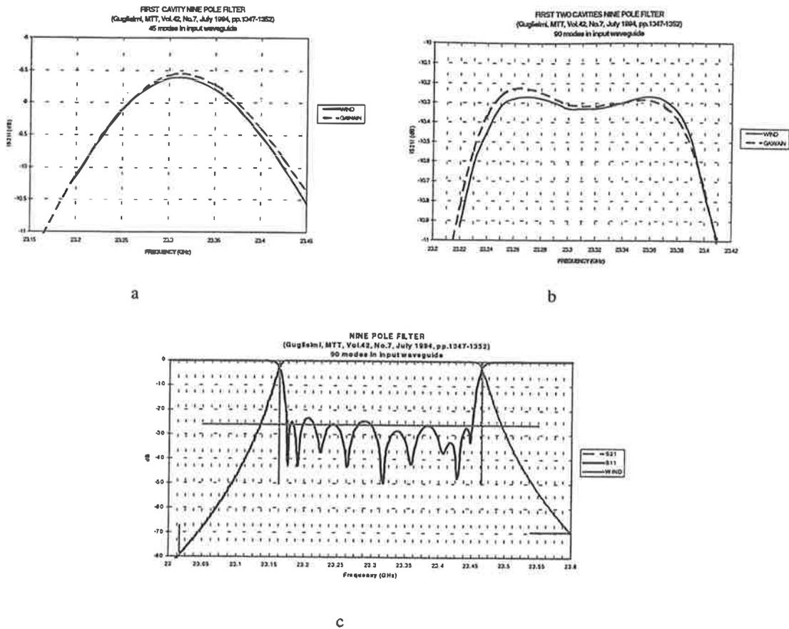
Figure 5: Simulation results nine-pole waveguide filter (Ref. 19)
