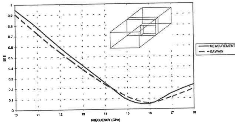
Figure 8: Reflection coefficient unsymmetric resonant iris with finite thickness
