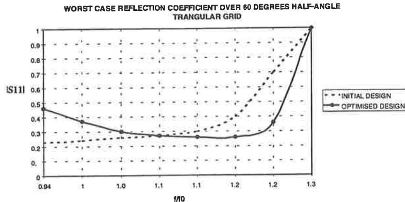
Figure 11: Result automated antenna synthesis
