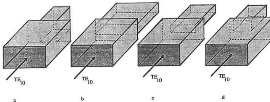
Figure 4: Waveguide step discontinuities
