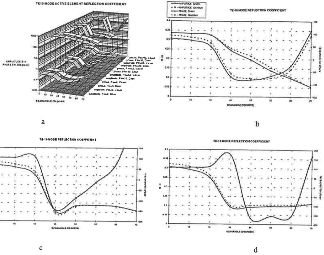
Figure 9: Active element reflection coefficient vs. scan angle for different scan planes
