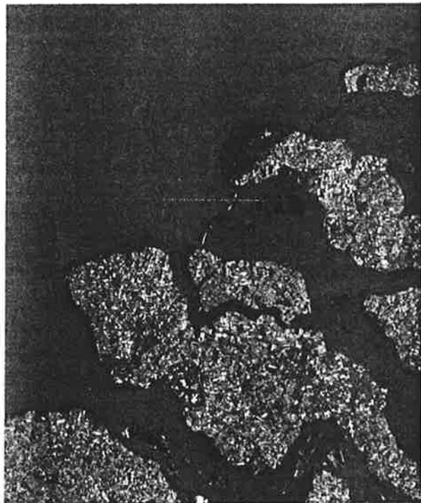
Figure 3. SAR intensity image (left) and phase-difference image (right) of Zeeland, the Netherlands, generated with the interferometric SAR processor of TNO Physics and Electronics Laboratory, the Netherlands, using repeat-pass ERS-1 imagery.
