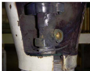
Typical oxygen incident outcome - damaged equipment.
