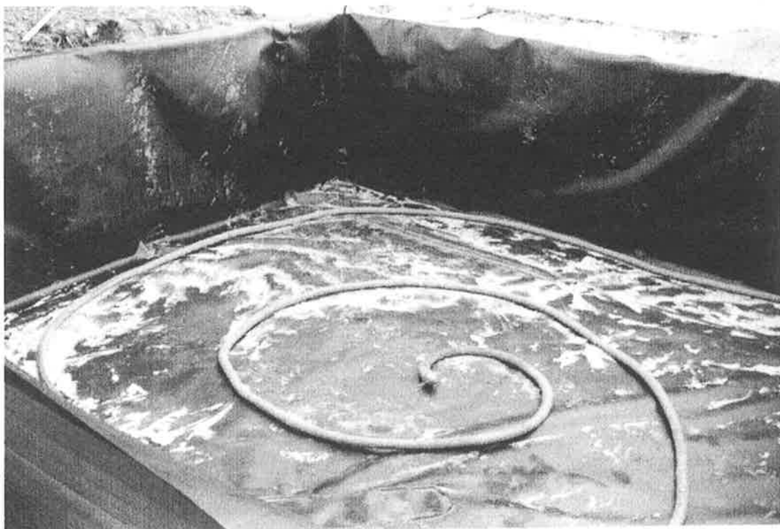
Figure 3.9 Installation of the drainage system in the wooden box.
