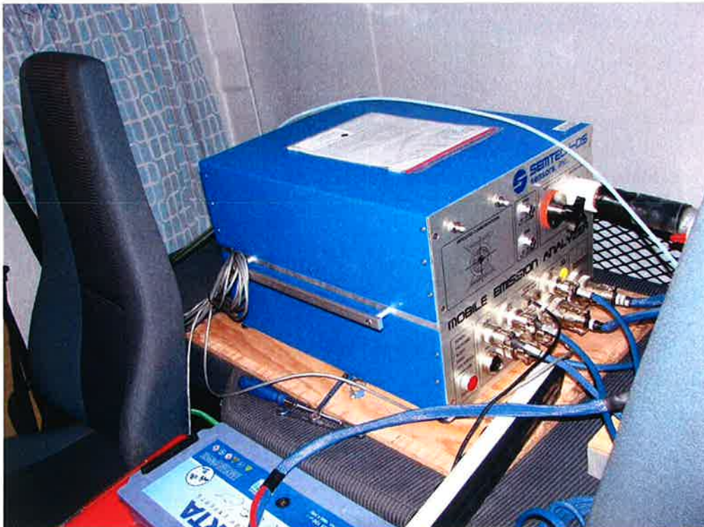
Figure1; PEMS main unit (SEMTECH DS) installed in a HD vehicle and PEMS EFM II attached to the exhaust.
