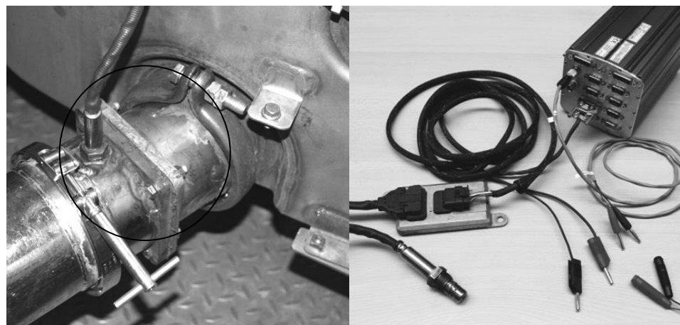
Figure 11 and Figure 12: left the NO x - O 2 sensor installed at the tailpipe of a Euro VI heavy-duty vehicle. Right, the sensor and data-acquisition unit which logs the sensor data, GPS data and optionally the CAN data.
