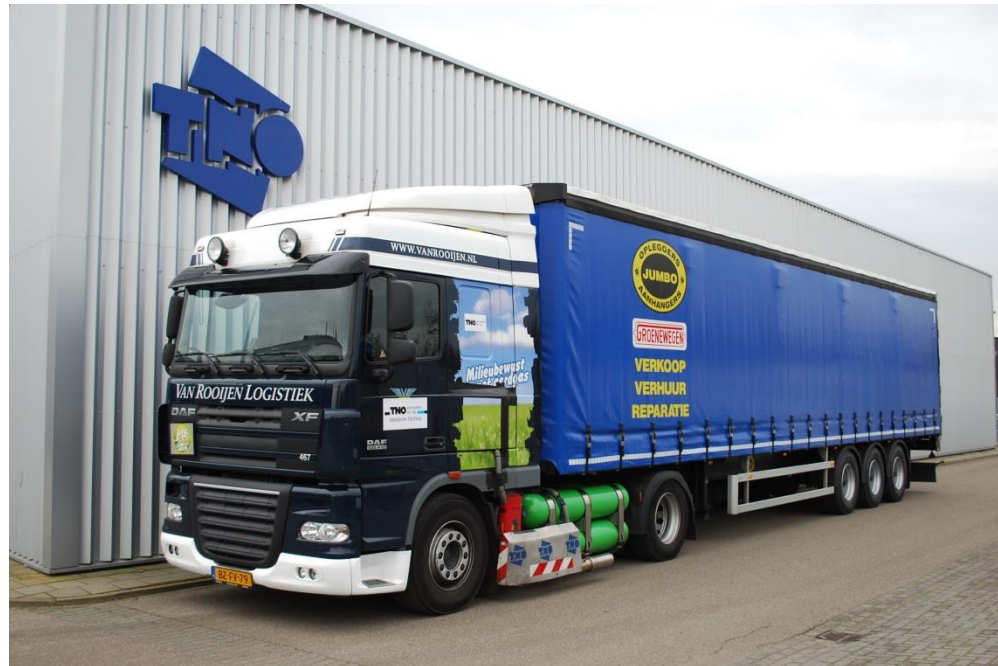
Figure 7: test vehicle for the PEMS measurements on a truck equipped with a retrofit dual-fuel system, running on diesel and compressed natural gas.
