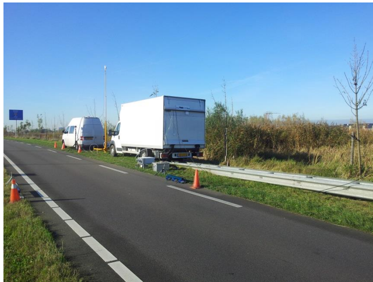
Figure 10: RES test set-up with the additional sniffer pole, measuring \text{NO}_x and \text{CO}_2 .
