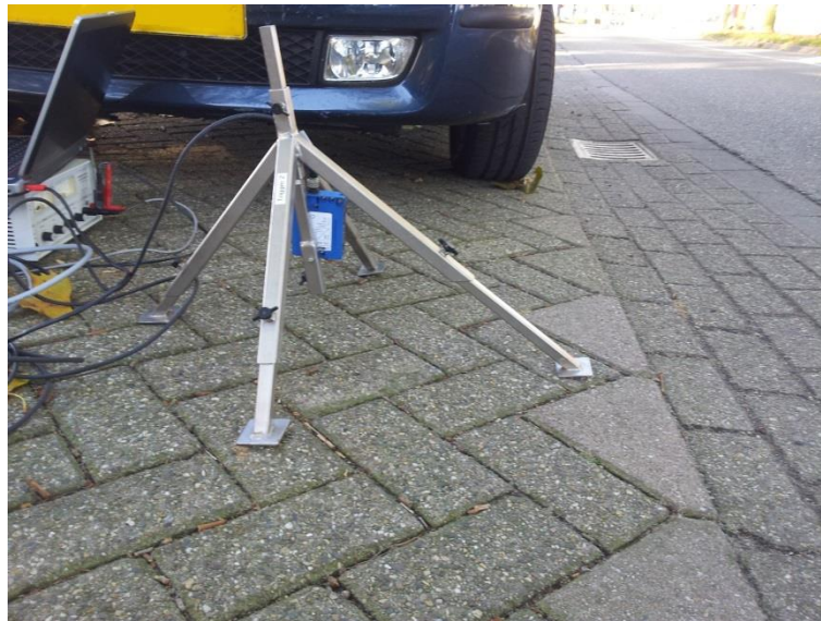
Figure 9: optical gate able to count the number of axles of a vehicle passing by.
