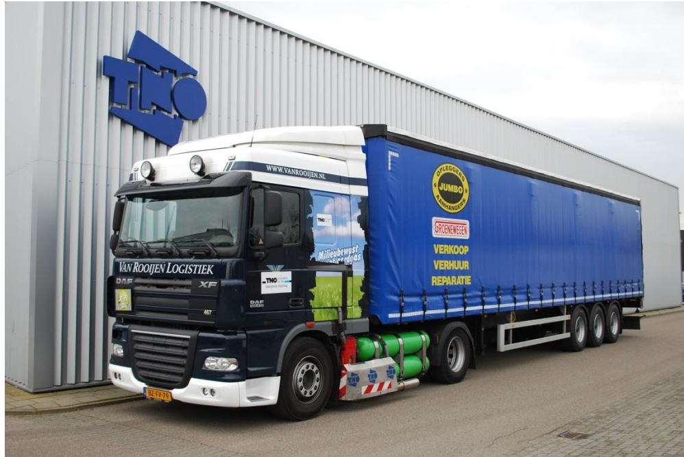
Figure 8: test vehicle for the PEMS measurements on a truck equipped with a retrofit dual-fuel system, running on diesel and compressed natural gas.
