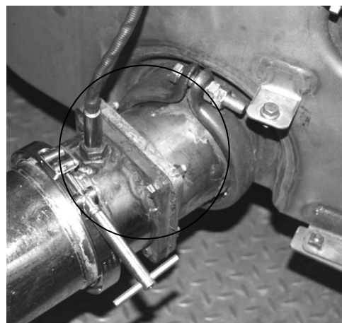
Figure 12: The NO x - O 2 sensor installed at the tailpipe of a Euro VI heavy-duty vehicle.
