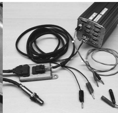
Figure 13: The sensor and data-acquisition unit which logs the sensor data, GPS data and optionally the CAN data.
