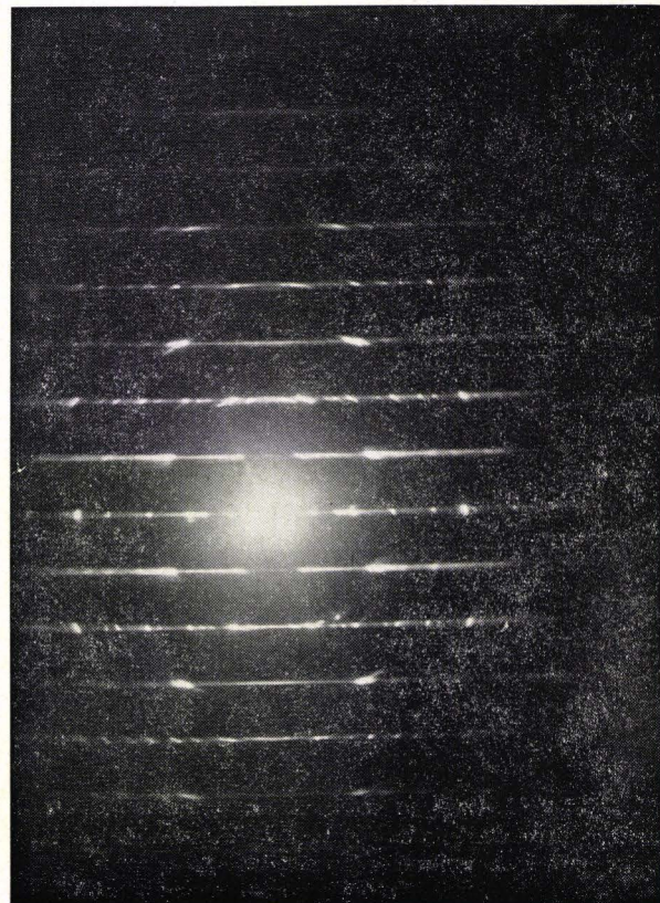
Fig. 7b. Electron diffraction pattern of the same fiber.
