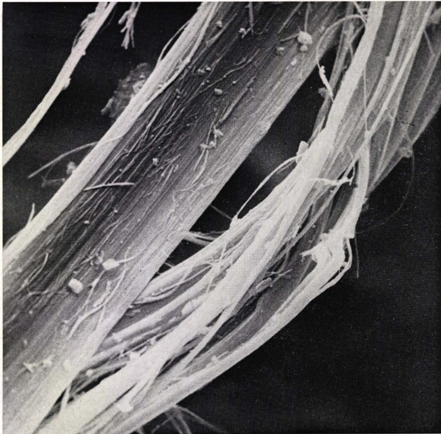
Fig. 1. Chrysotile asbestos fibers (2750 × C.E.M. Central Lab. TNO).
