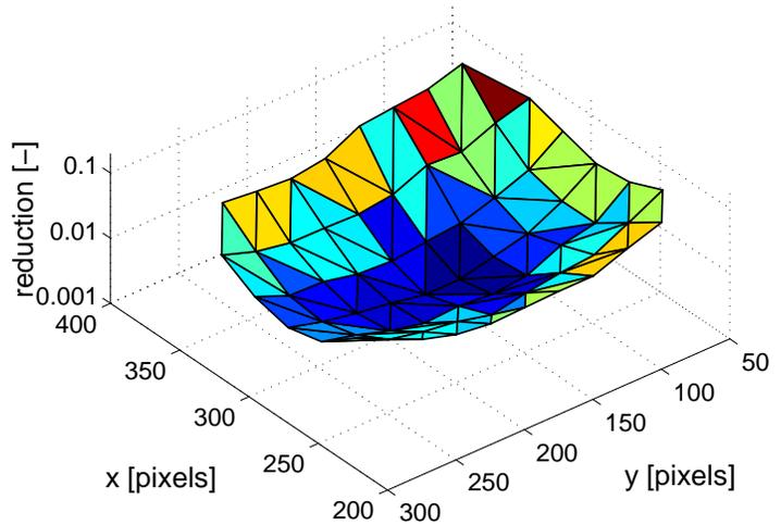
**Figure 2.** Reduction of the mean square wavefront prediction error  $J_2^{KP}(j)/J_2^{RW}(j)$  over the aperture.
