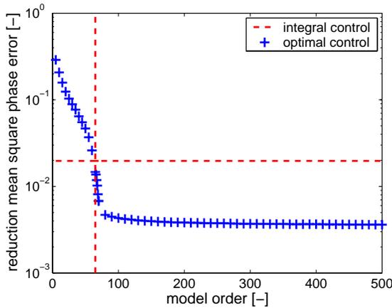
**Figure 3.** Normalized mean square wavefront prediction error  $J_1$  as a function of the model order. The dashed lines correspond to the performance and equivalent model order of the random walk predictor (18).
