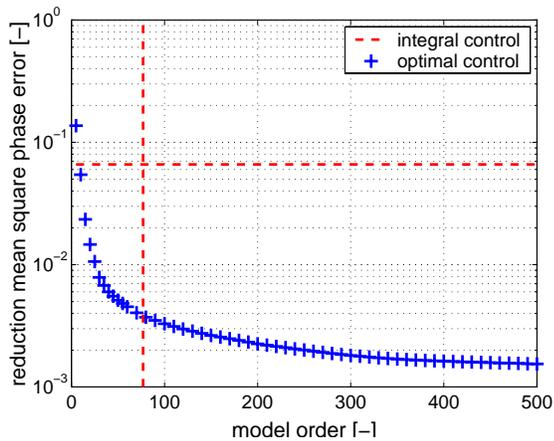
**Figure 1.** Normalized mean square wavefront prediction error  $J_1$  as a function of the model order. The dashed lines correspond to the performance and equivalent model order of the random walk predictor (18).
