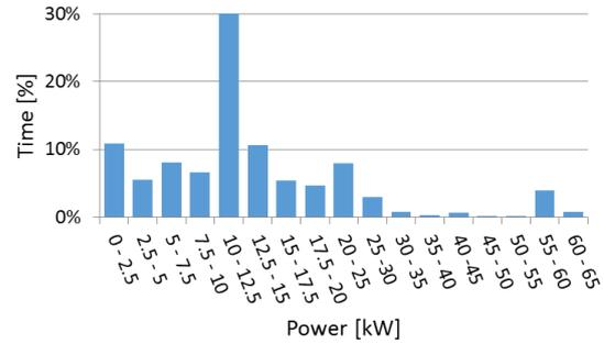
Figure 1: Operational profile of the canal boat
