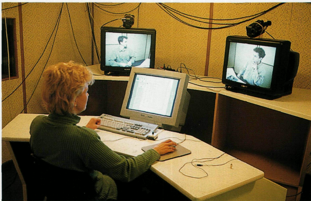
Experimental set-up for the investigation of advantages and disadvantages of video conferencing. In some respects video conferencing is improved by selective gaze.
