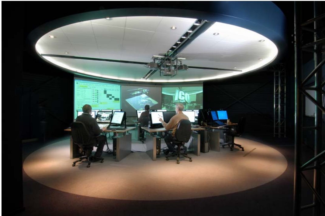
Figure 5: ICO: Integrated Command Environment for the Bridge, Command Centre and Engine Room of a Frigate.
