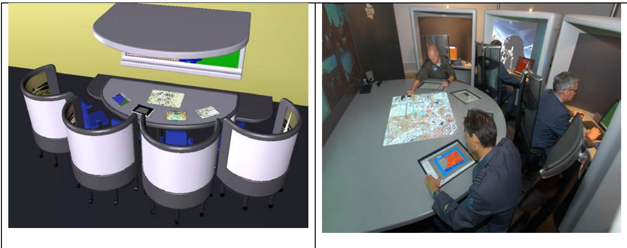
Figure 7: CH: Cannibal Hector, a Joint Operating Centre for the Supreme Staff. The left panel depicts an early CAD-model showing the basic lay-out of four "cubicles" draped around a central workspace. The panel on the right is a photograph of the current situation. Two of the four commanders are working in their personal workplaces, interacting with staff members at a reachback position. Also see figure 3.
