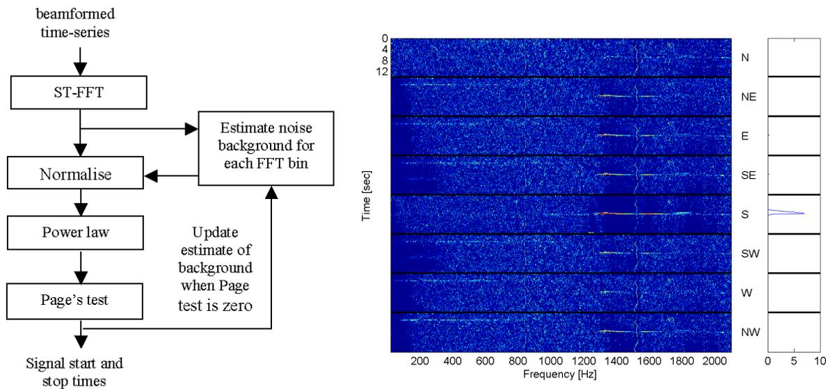
*Fig. 1: On the left the schematic of the detector and on the right the detector display, which is a multi-beam LOFAR of the normalised data (left) and corresponding Page-test output (right). The blue line on the right side depicts the Page-test output and marks a short signal detection in the Southern (aft) direction.*
