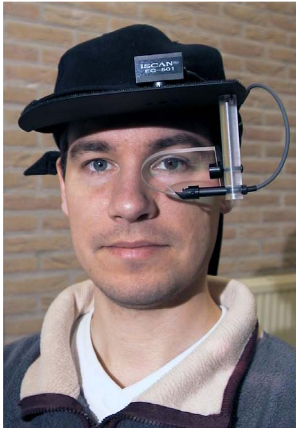
Fig. 6. Participant wearing baseball cap with pupil size measurement equipment.
