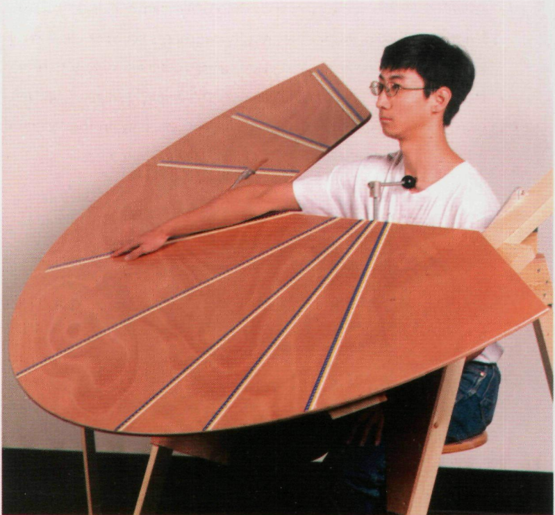
Figure 2. Subject sitting at the experimental workstation for testing the validity of the skeleton of digital human models through maximum reach measurements.
