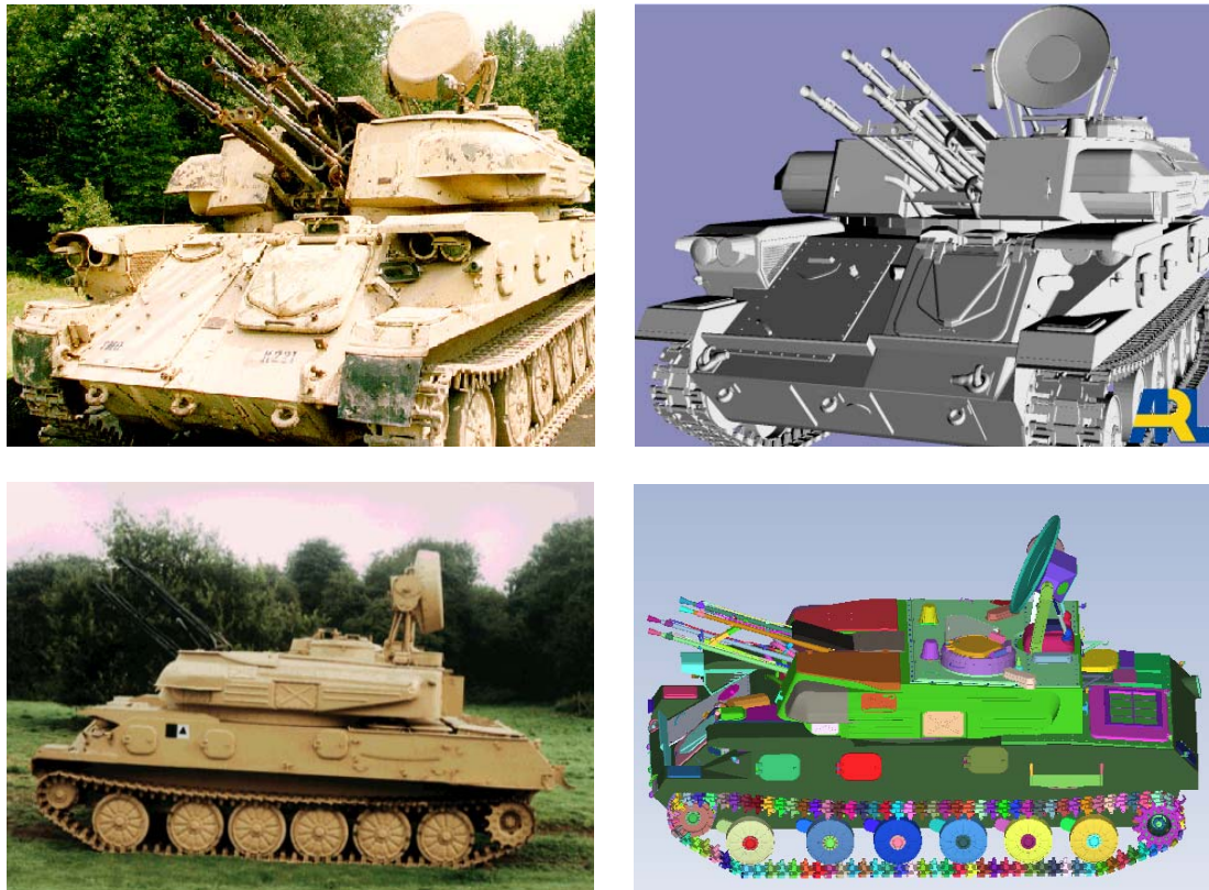
Figure 1. Picture of the ZSU-23 (left) and the high fidelity facet model (right) of the ZSU23-4 used by the calculations. The different facets are indicated by various colours in the lower-right frame.
