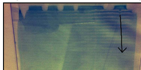
Figure 6 Barring in a coated layer. Arrow is coating direction.
