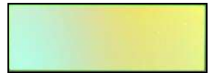
Figure 3 An OLED with not uniform functional layer thickness.
