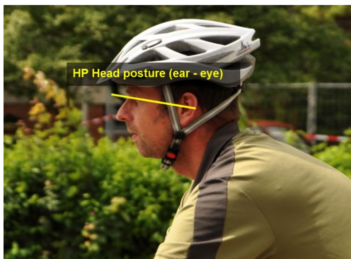
Figure 37: Establishment of the head posture angle by measuring the inclination of the line from the ear to the eye.
