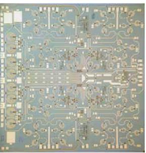
Figure 18 Ku-Band 8-Channel Downconverter
