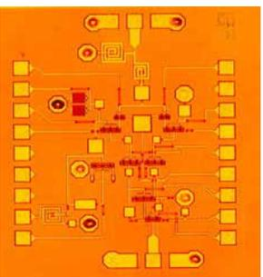
Figure 12 X-Band active tunable filter
