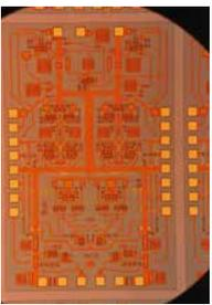
Figure 9 Differential Vector Modulator
