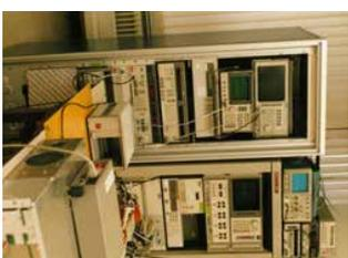
Figure 4 HP8510B measurement setup
