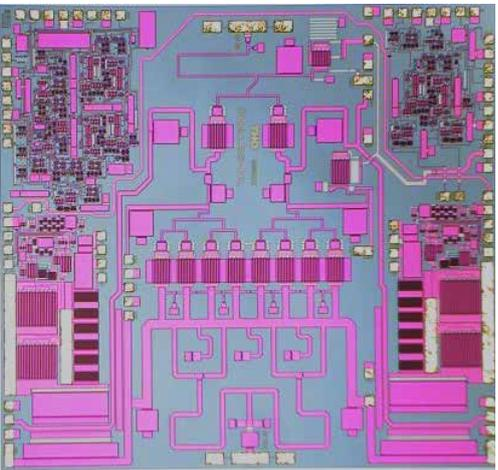
Figure 21. Integrated power amplifier and power supply
