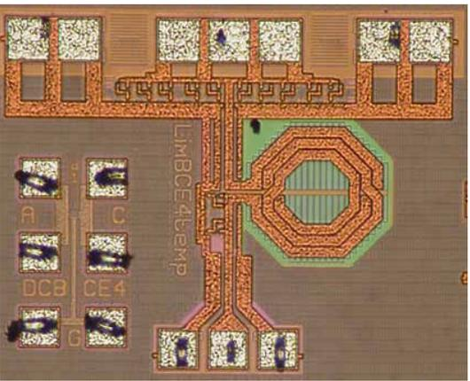
Figure 25 First integrated Sige limiter in 0.25 μm BiCMOS
