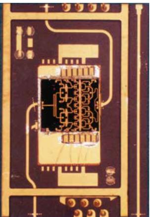
Figure 10 5 Watt GaAs HPA in ceramic package
