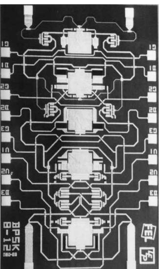
Figure 6 First BPSK phase shifter, the basis for the first vector modulator
