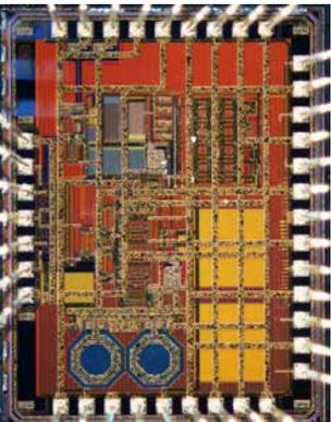
Figure 23 SiGe type-II PLL for integrated radar chip generation
