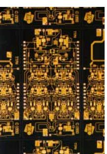
Figure 8 First MMIC vector modulator, based on the BPSK modulators
