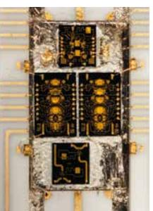
Figure 7 Hybrid vector modulator employing two BPSK phase shifters, an active 90 degrees splitter and a passive combiner
