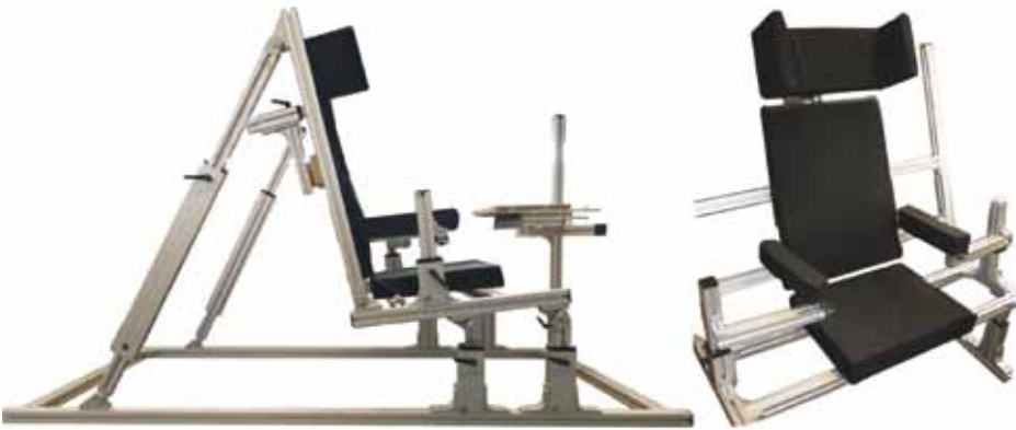
Figure 6.3 Adjustable research seat for the long-term experiment
