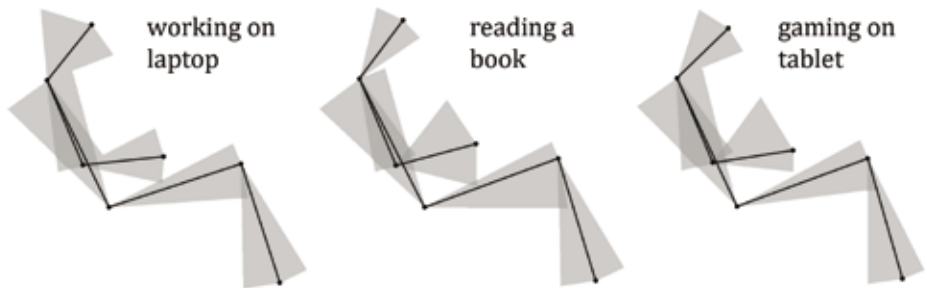
Figure 3.4 Observed body angles observed from the side for three activities; black lines are mean values for each task, grey areas indicate the variation between minimum and maximum angle.
