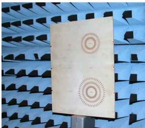
Figure 3: Panel with six antennas located in a square grid
