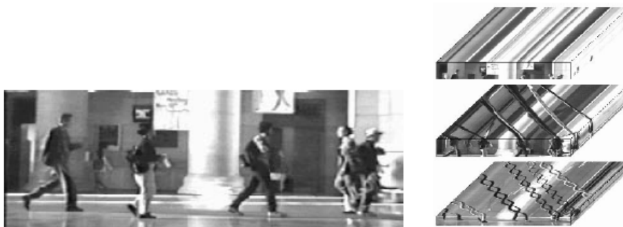
Figure 2.3: On the left one frame of an image sequence is shown, on the right a number of xt -slices from the xyt -cube. The recurrent leg motion of a walking human can clearly be seen. From [Niyogi and Adelson, 1994].
