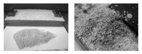
Figure 4: Sanding of the outer layer of the lime-cement mortar in the presence of NaCl after 6 RH cycles
