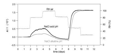
Figure 9: Dilation of specimens contaminated with acid and alkaline NaCl solution during a RH cycle
