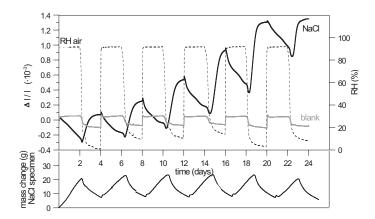
Figure 3: Dilation of blank and NaCl contaminated specimens (upper graph) and weight change of NaCl contaminated specimen (lower graph) during RH cycles
