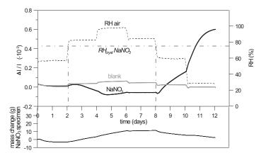
*Figure 7: Dilation of blank and NaNO*<sub>3</sub> *contaminated specimens (upper graph) and change in weight of the NaNO*<sub>3</sub> *contaminated specimen (lower graph) during a RH cycle*
