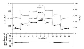
Figure 6: Dilation of blank and NaCl contaminated specimens (upper graph) and weight change of NaCl contaminated specimen (lower graph) during a RH cycle below 75%RH
