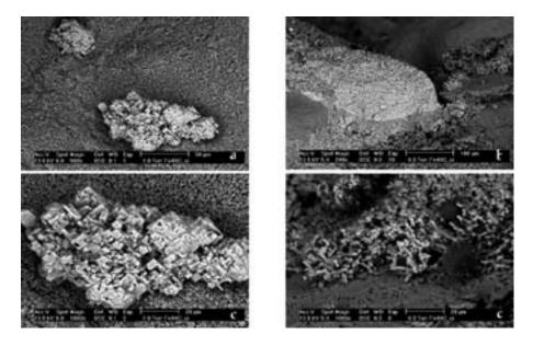
*Figure 16: ESEM photomicrograph showing NaCl crystallization in presence of inhibitor; crystal agglomerations (white areas) are observed (a-b); the crystal may be more (c) or less regular (d)*
