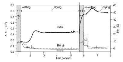
*Figure 2: Dilation of blank and NaCl contaminated specimens during wetting at RH=50% (gray areas) and drying at 0%RH (white area) cycles*
