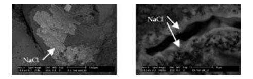
*Figure 14: ESEM photomicrographs showing NaCl (lighter areas) crystallizing as a layer in specimens contaminated with acid (left) and alkaline (right) NaCl solution*
