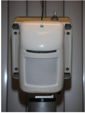
Figure 2. One PIR sensor and camera wireless node mounted on posts.
