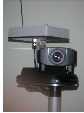
Figure 2. One PIR sensor and camera wireless node mounted on posts.
