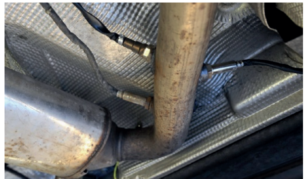
The SEMS system includes one or two \text{NO}_x sensors and an \text{NH}_3 sensor, which can be easily attached to the exhaust of a vehicle.
