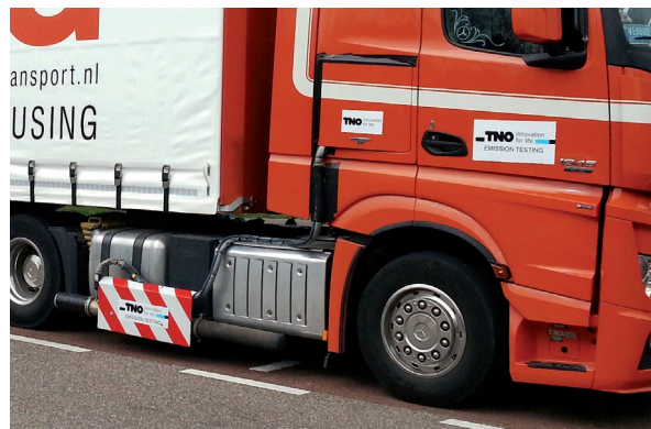
The PEMS system installed on a Euro VI long-haul commercial vehicle.
