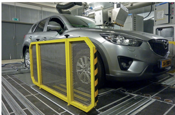
Chassis dynamometer Horiba Oberursel, 2011.
