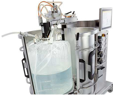
Single-use reactor bags in biotechnology (Sartorius Stedim Biotech S.A.)
