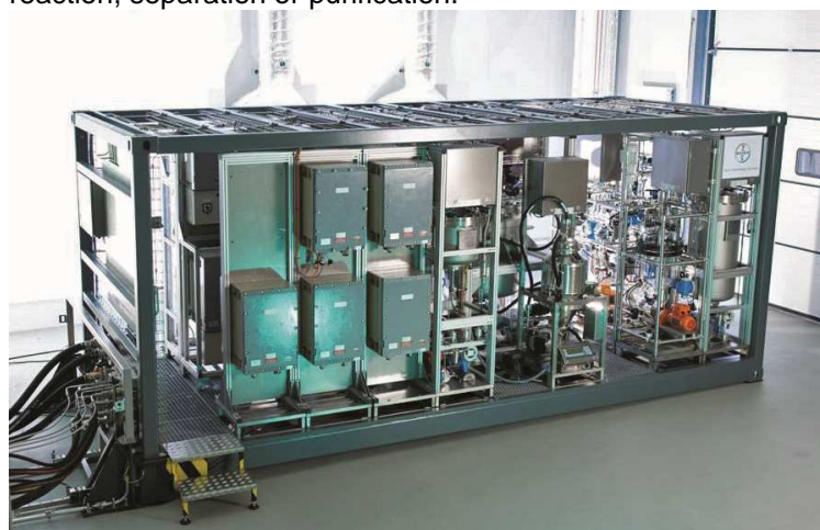
Bayer's Process Equipment Container Unit installed at INVITE
