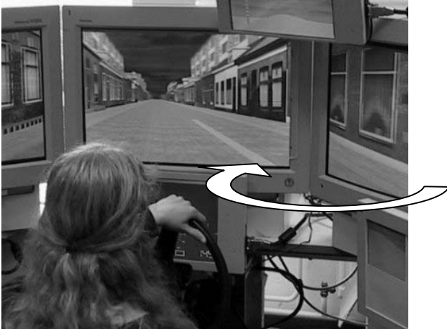
Figure 14. The arrow points to an augmented instruction which is presented on the central screen of the LOCS. A bar (protruding from the virtual car) has appeared. It indicates a lateral position too far to the left; hence, the driver should steer right (towards the bar) to try to align the bar to the curb. It can be seen that the ideal lateral position of the car is with the curb aligned to the lower right corner of the windshield (i.e. the central screen).
