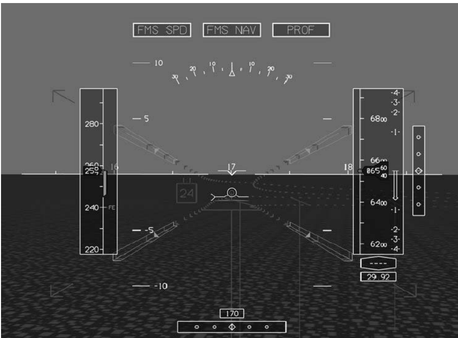
Figure 3. Augmented cues in use in an aircraft display. The so called 'highway in the sky' helps aircraft pilots during descent by depicting a flight path on a display.
