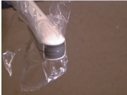
Figure 5. A method to ensure that the thermocouple is in firm contact with the transducer surface, without affecting the accuracy of the measurement.
