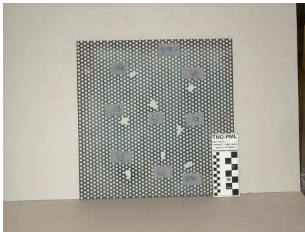
Fig. 11. Frontside of a front plate of MARS-300 perforated, armour configuration 11.
