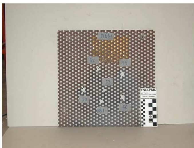
Fig. 14. Frontside of a plate of MARS-300 perforated, armour configuration 12 (60° NATO).
