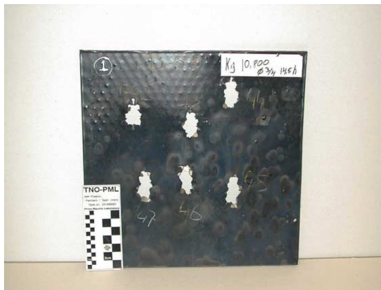
Fig. 21. Frontside of a LIBA plate of armour configuration 10, impacted at 60° NATO.
