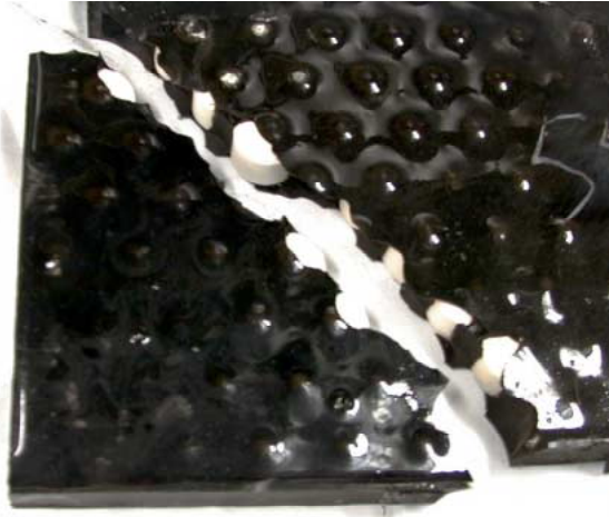
Fig. 20. Part of a LIBA plate of armour configuration 9, showing its composition.
