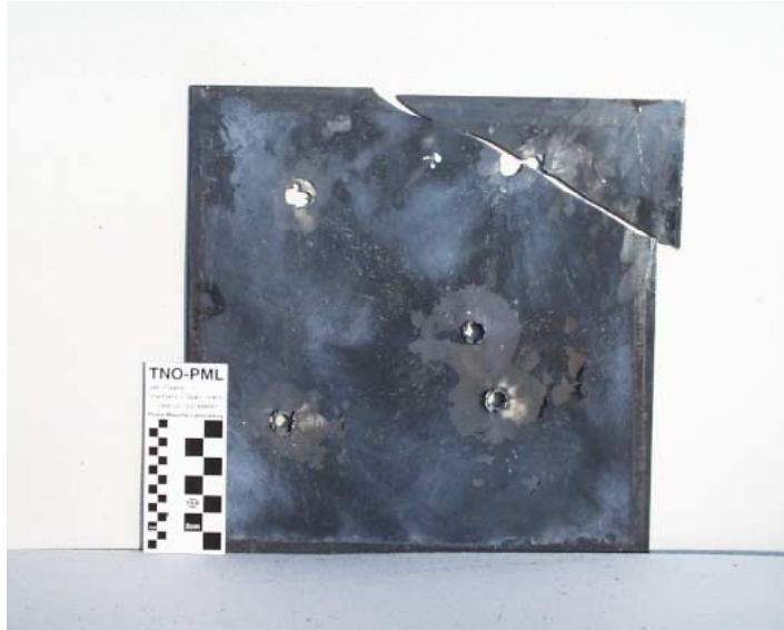
Fig.8. Crack in corner of SPS-43 steel armour plate (armour configuration 1).
