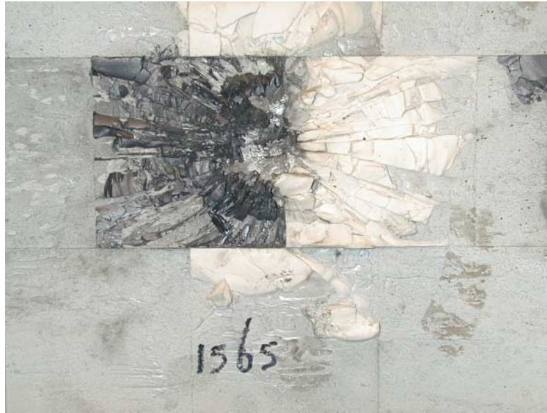
Fig. 23. SiC tile (black), leaving the underlying aluminium armour undamaged.
