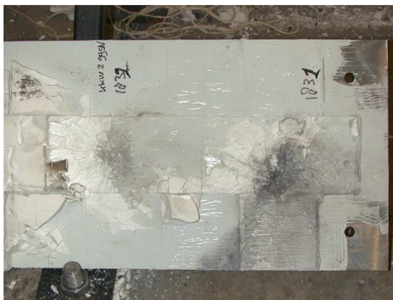
Fig. 24. 'Common' \text{Al}_2\text{O}_3 tiles on aluminium, stopping 14.5 mm AP-I B32.
