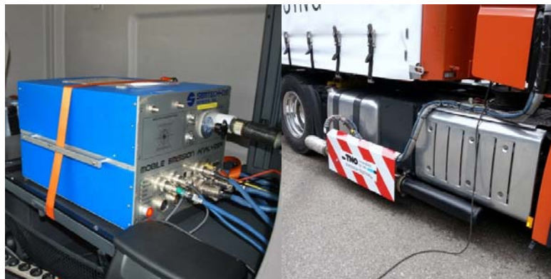
Figure 1: Two important PEMS parts: the integrated gas analysers and PEMS control unit (left) and the exhaust flow meter (right) mounted on the tail-pipe of a heavy-duty vehicle.
