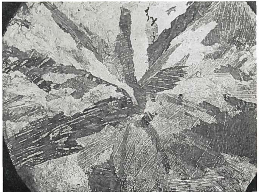
Fig. 1 Spongy-dendritic solidified brass, with 65,7% Cu and 0,26% Al. 12x
