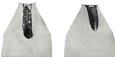
Fig. 3 Shrinkage cavity of a Tatur-cone with 68,0% Cu and 0,33% Al.
