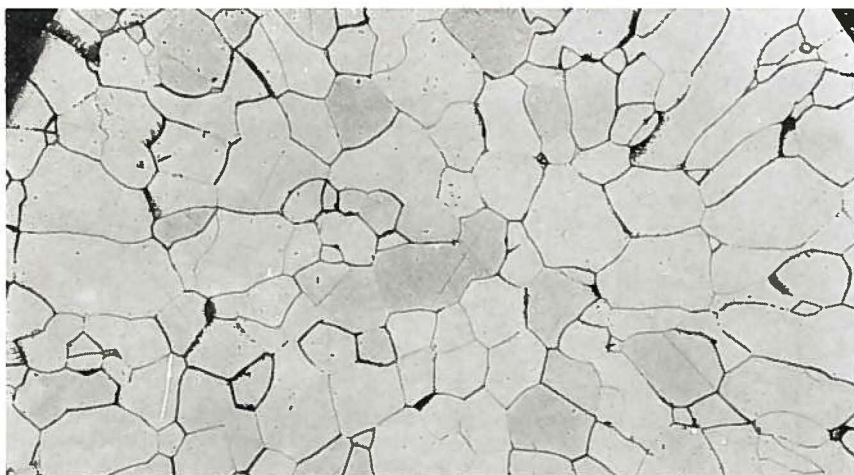
Fig. 2 Endogeneous compact solidified brass, with 56,1% Cu and 0,27% Al. 12x
