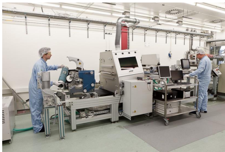
Figure 7. Holst Centre's R2R print line with rotary screen, inkjet stations and photonic curing unit (box in the middle).
