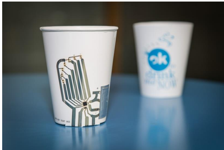
Figure 2. prototype of a temperature sensitive coffee cup with Printed Electronics (Holst Centre 2014)
