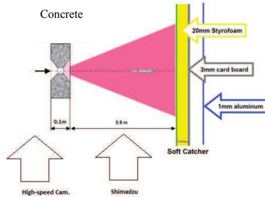
Figure 38 Test set-up ballistic experiments
