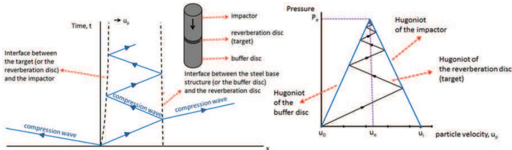
Figure 35 Impedance mismatch technique for linear elastic reverberation disc
