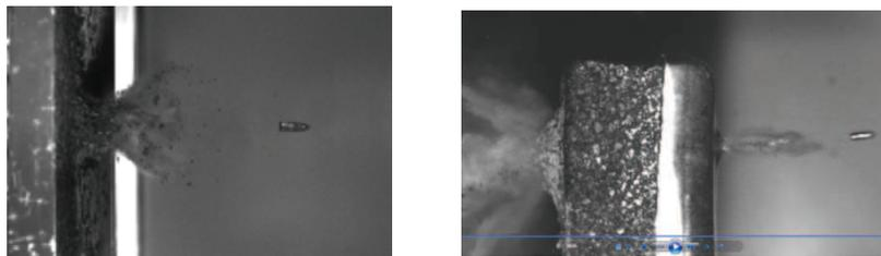
Figure 39 Ballistic tests. Left: porous concrete. Right: polymer filled porous concrete
