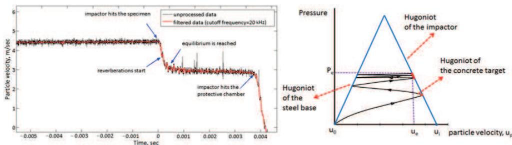
Figure 36 Particle velocity history - Impedance mismatch technique for reverberations in porous concrete
