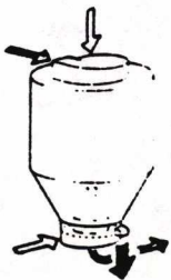
Co-current, with integrated fluid bed, rotary or nozzle atomizer, for dairy/food products.
