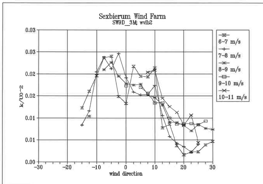
Figure 4.13 Turbulent kinetic energy  $k/U_0^2$  as a function of wind direction at sensor b2
