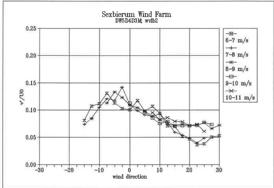
Figure 4.11 Lateral turbulence intensity  $v'/U_0$  as a function of wind direction at sensor b2
