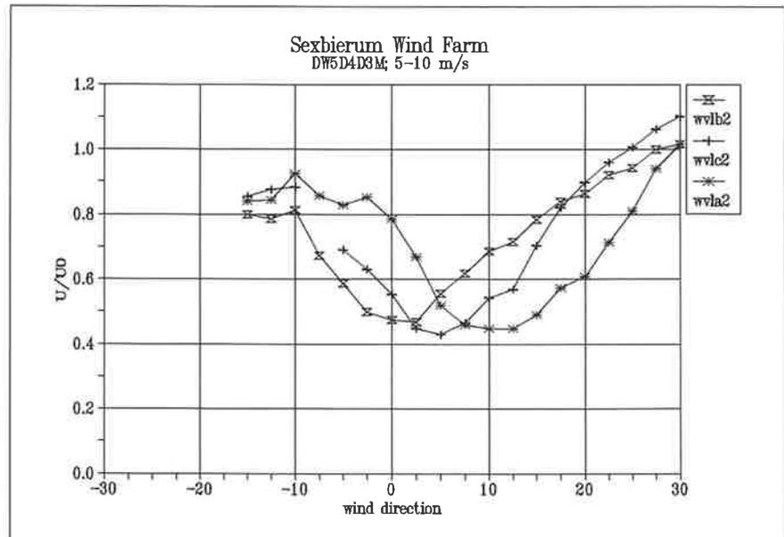
Figure 4.7 Wind speed ratio  $U/U_0$  as a function of wind direction for sensors b2, c2 and a2
