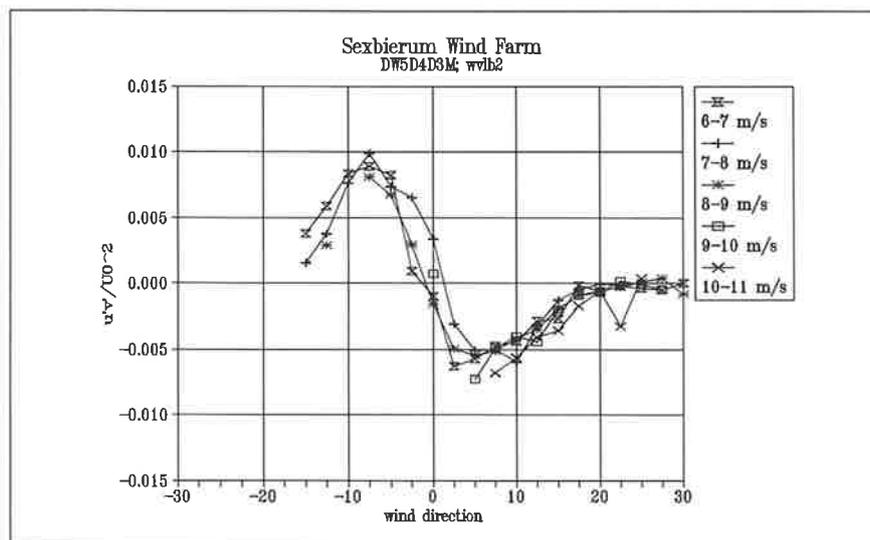
Figure 4.17 Shear stress  $u'v'/U_0^2$  as a function of wind direction at sensor b2
