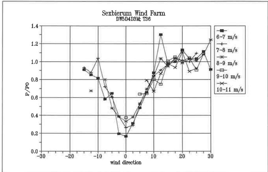
Figure 4.3 Power ratio of turbines T36 with respect to turbine T38
