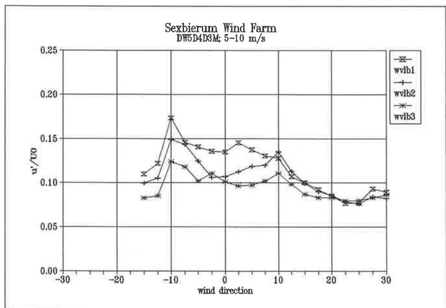
Figure 4.15 Aggregated turbulence intensity  $u'/U_0$  as a function of wind direction at mast b
