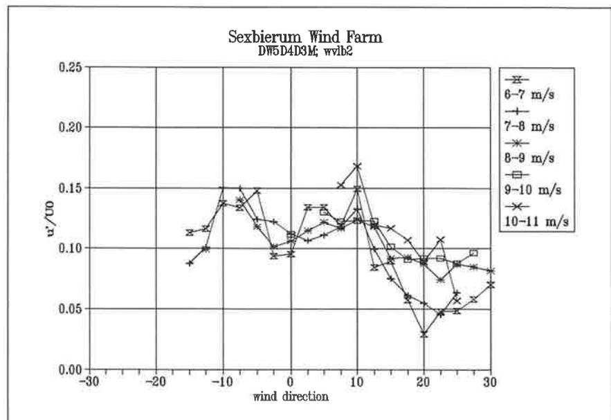
Figure 4.10 Turbulence intensity  $u'/U_0$  as a function of wind direction at sensor b2
