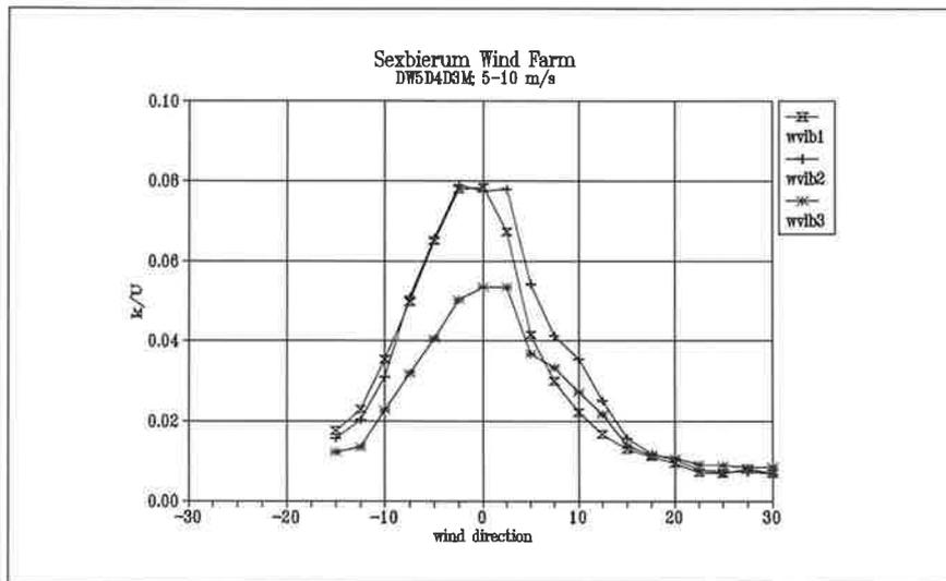
Figure 4.16 Turbulent kinetic energy non-dimensionalized with local velocity as a function of wind direction
