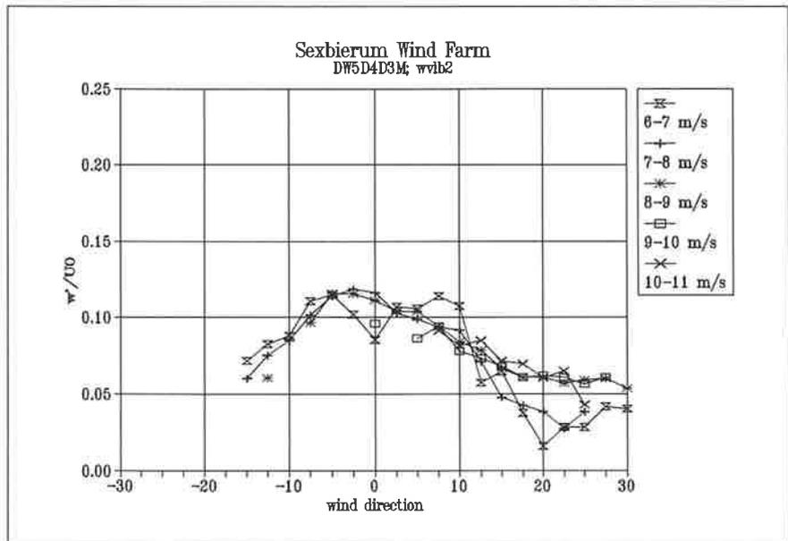
Figure 4.12 Vertical turbulence intensity  $w'/U_0$  as a function of wind direction at sensor b2
