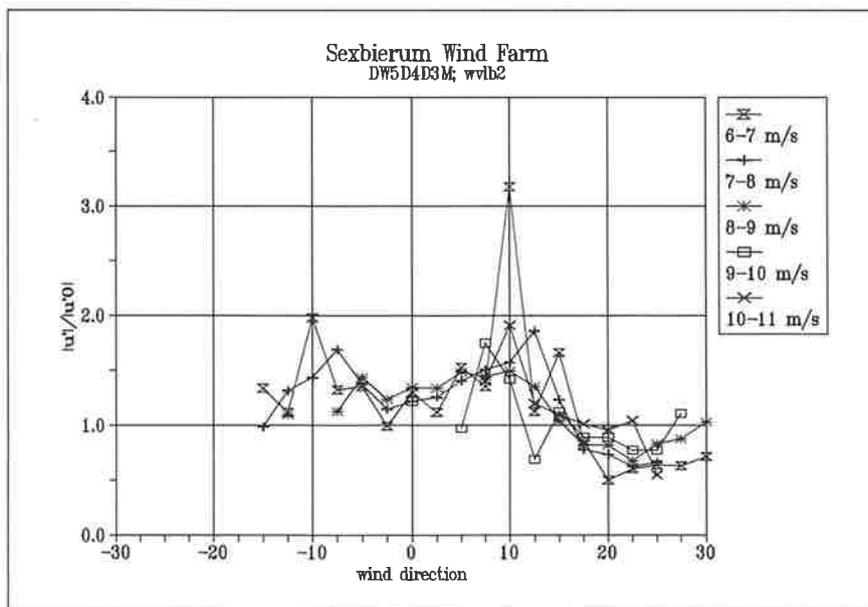
Figure 4.14 Ratio of wake turbulence and undisturbed turbulence  $u'/u_0'$  as a function of wind direction at sensor b2
