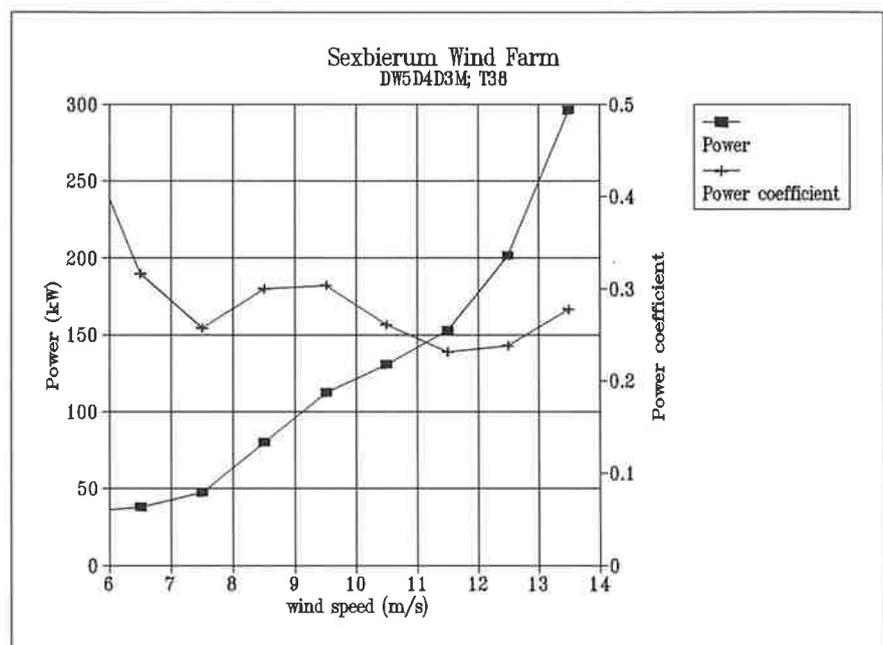
Figure 4.2 Power curve and power coefficient of wind turbine T38, based on 3-minutes averages
