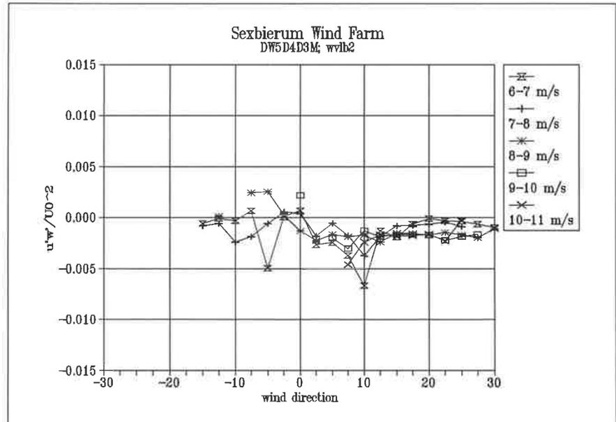
Figure 4.19 Shear stress  $u'w'/U_0^2$  as a function of wind direction at sensor b2
