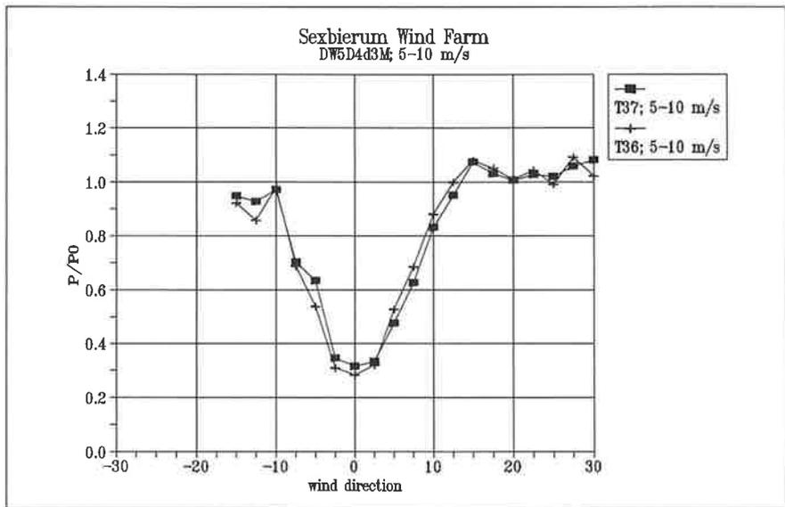
Figure 4.4 Aggregated power ratio of turbines T36 and T37 with respect to turbine T36
