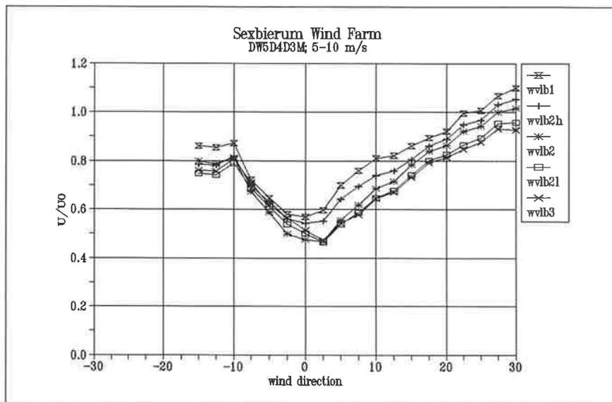
Figure 4.8 Wind speed ratio  $U/U_0$  as a function of wind direction for sensors b1, b2h, b2, b2l and b3
