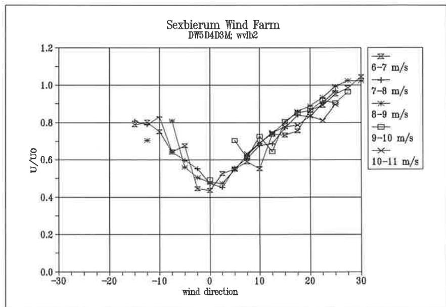
Figure 4.5 Wind speed ratio  $U/U_0$  at sensor b2 as a function of the undisturbed wind direction
