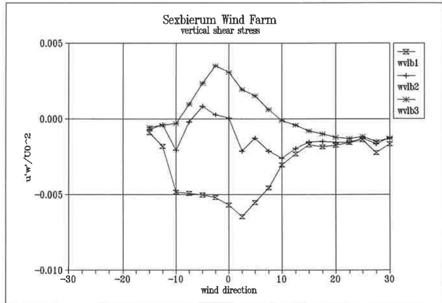
Figure 4.21 Shear stress  $u'w'/U_0^2$  as a function of wind direction for sensors b1, b2 and b3
