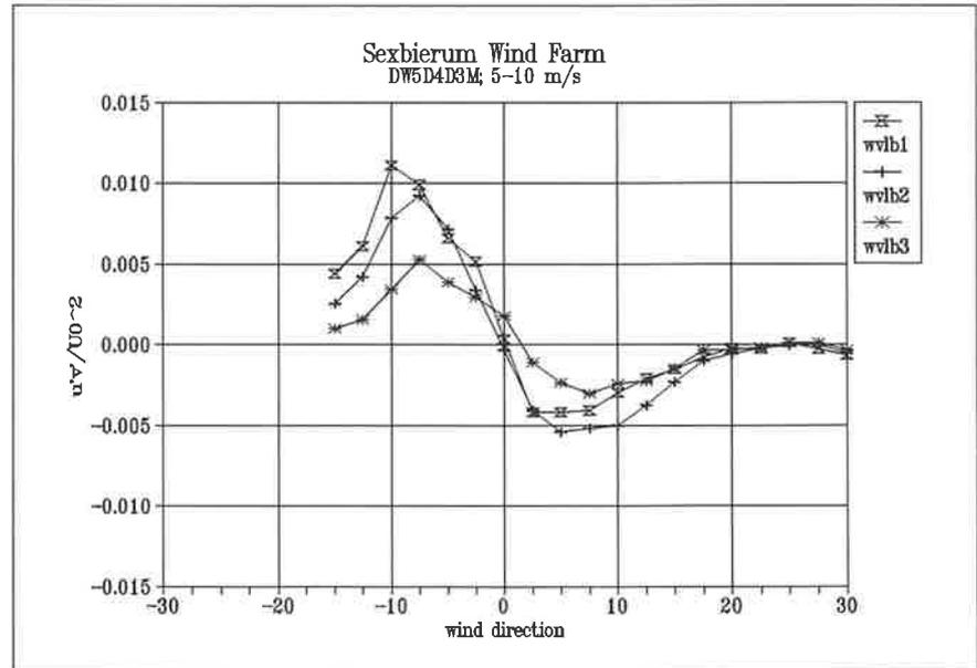
Figure 4.20 Shear stress  $u'v'/U_0^2$  as a function of wind direction for sensors b1, b2 and b3
