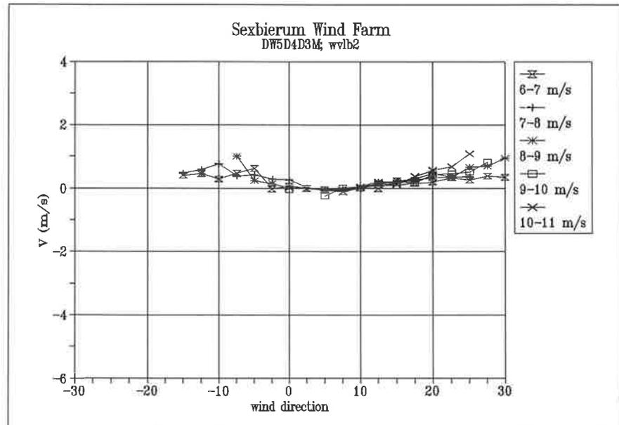
Figure 4.6 Lateral wind speed  $V$  as a function of wind direction
