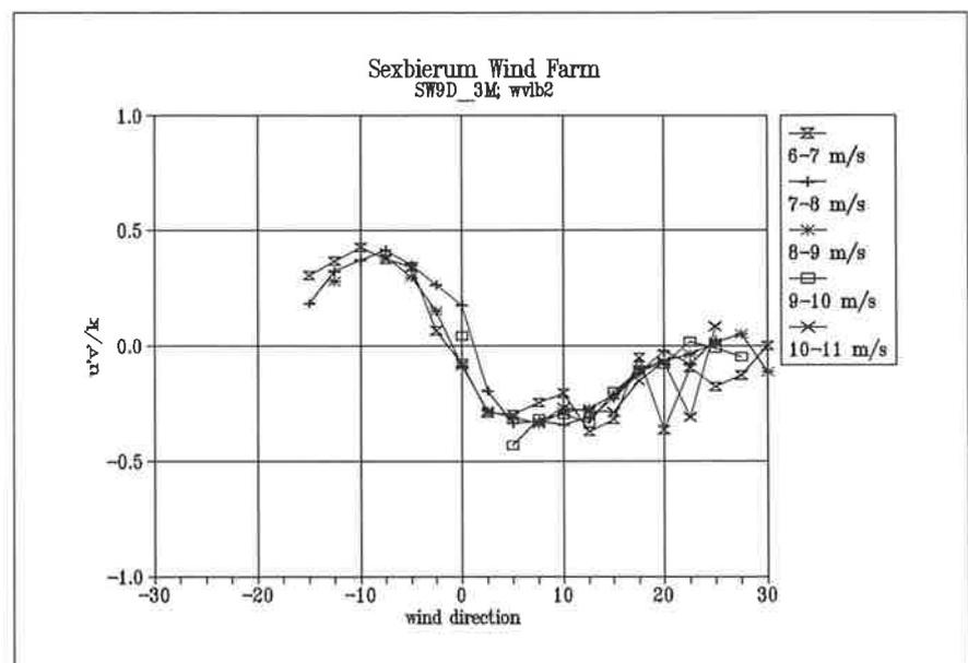
Figure 4.18 Shear stress  $u'v'$  non-dimensionalized with the local turbulent kinetic energy as a function of wind direction at sensor b2
