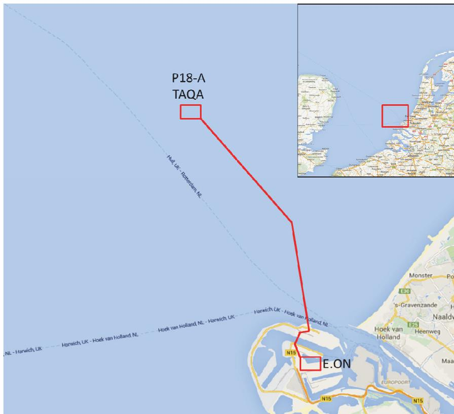
Fig. 1. Approximate lay-out of the ROAD CCS project. The EON power plant is located in the Rotterdam harbor area ('E.ON'); the transport pipeline is indicated in red; the storage location is the P18-4 depleted gas field; the platform is located in the red box labelled 'P18-A'.
