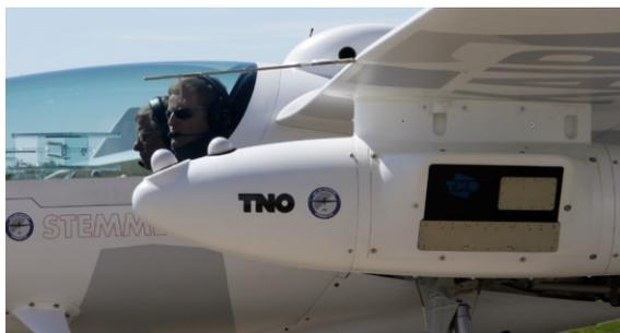
**Figure 6:** AMBER installed in a pod for flights on a motor glider. On the front, two GPS antennas are mounted.
