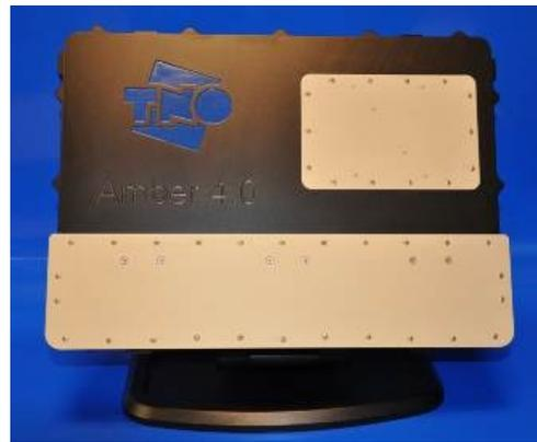
**Figure 1:** Photograph of the Affordable Multi-beam Radar (AMBER) System front side. The 8 element reconfigurable transmit antenna is in the upper right corner. The 24 element receiver patch array is at the bottom.
