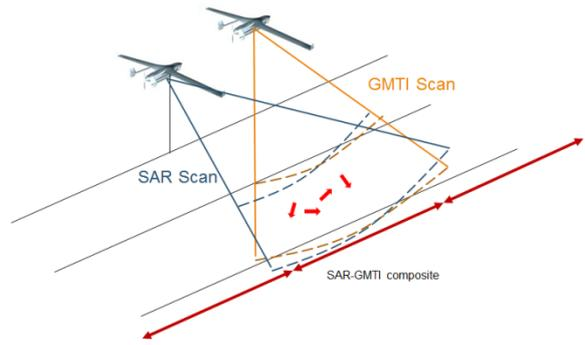
**Figure 4:** Simultaneous STRIP-SAR and GMTI by time division, with continuous coverage.
