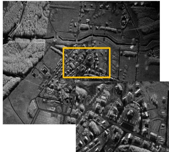
**Figure 7:** Example of a STRIP-SPOT mode: a 70 Mpixel image at high resolution. The box demarcates the approximate size of a conventional single-beam SPOT image at this resolution.
