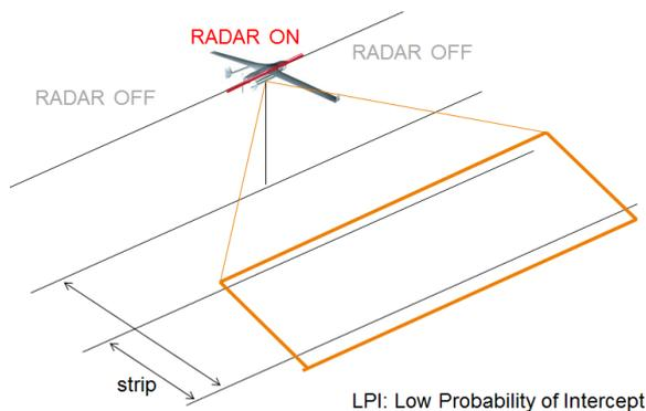
**Figure 5:** Example of a covert or LPI SAR mode.
