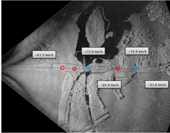
**Figure 9:** Wide area simultaneous SAR-GMTI image with moving targets projected at their actual positions on the road.
