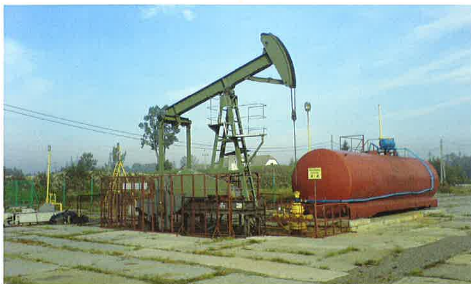
Figure 4. The well in Kaniów that was used as CO 2 injection well and that is used as production well in the MOVECBM project.
