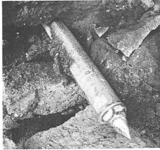
Fig. 18: A PUR-coated pipe after driving through a railway embankment
