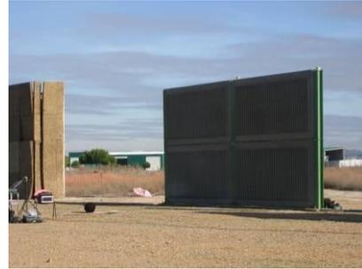
**Figure 65 - Barrier 1: Flat absorptive concrete (A2)**
