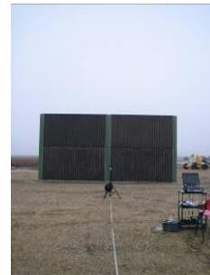
**Figure 66 - Barrier 2: Non flat absorptive concrete (A3)**
