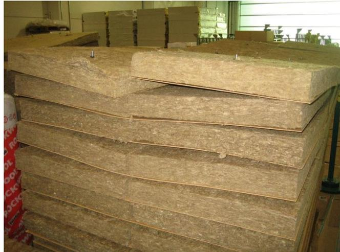
**Figure 41 - Rock wool panels manufactured to cover NRDs in WP2 measurements**
