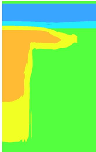
Figure 16. Test case: the yellow and orange surface show the area of the thermal crack in the reservoir and caprock (positive stresses in Figure 15 (right)).
