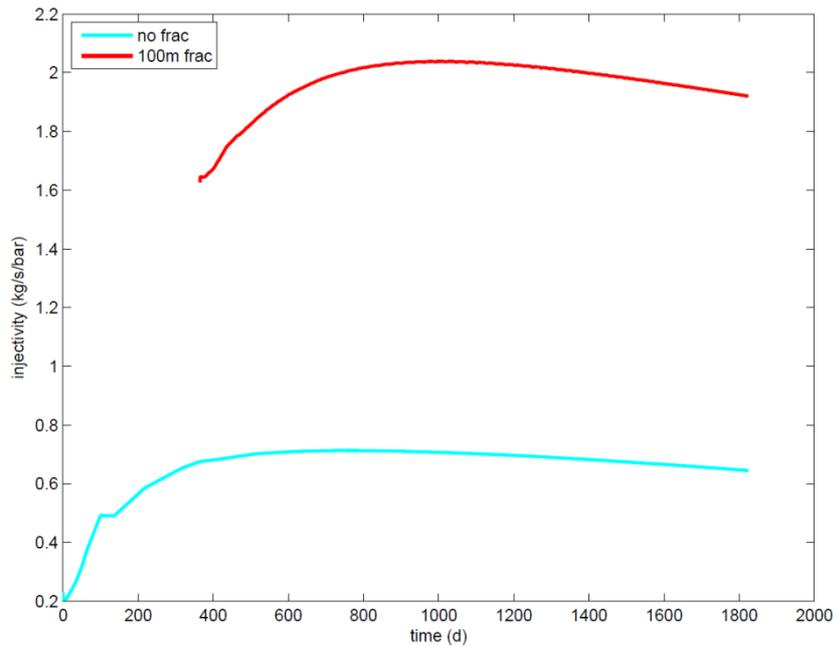
Figure 9. Injectivity with and without a fracture.
