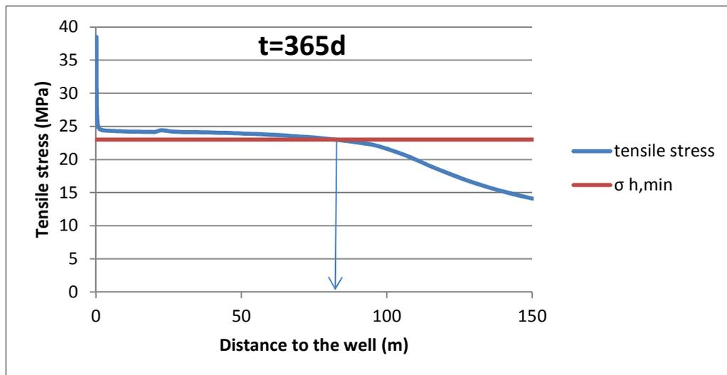
Figure 7. Tensile stresses with distance from the well after 365 days after the start of injection with  $\sigma_{h,min}=23$ MPa (red line).
