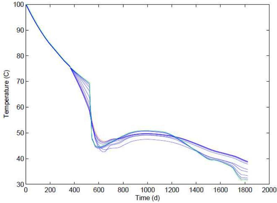
Figure 19. Temperature development over time in the fracture. Every line represents one grid block. The red line is the grid block closest to the well and the green line is the grid block at the end of the fracture.
