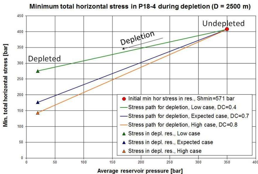
Figure 5 Value of the horizontal stresses for the undepleted and depleted reservoir at a depth of 2500 m [3].
