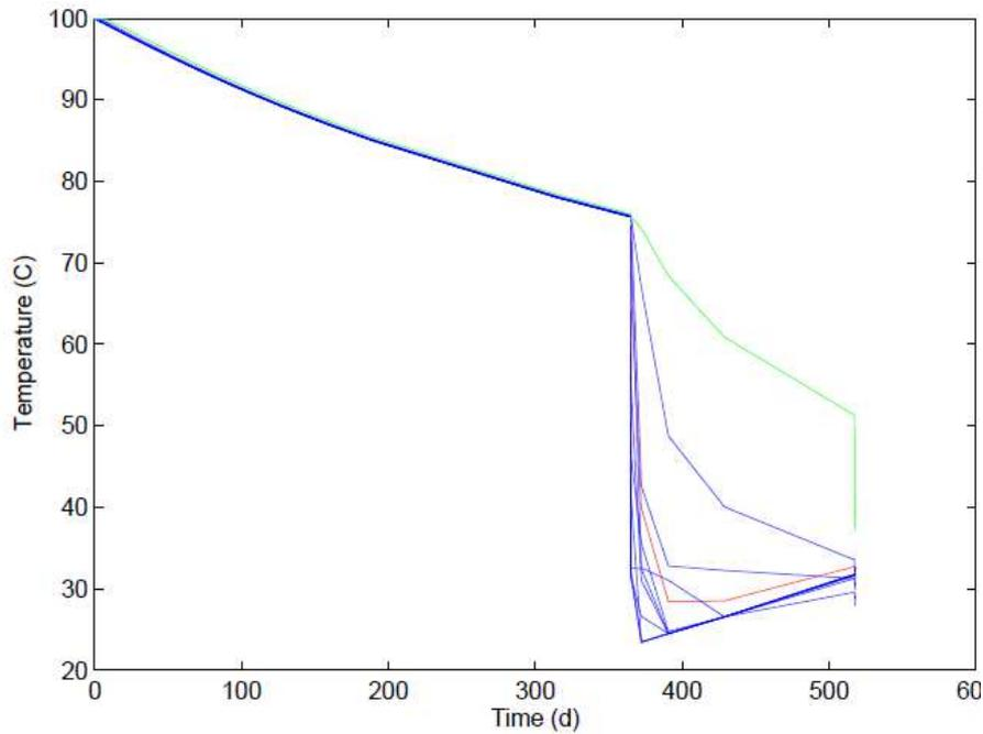
Figure 20. Temperature development over time in the fracture. Every line represents one grid block. The red line is the grid block closest to the well and the green line is the grid block at the end of the fracture for the case with decreased fracture permeability.
