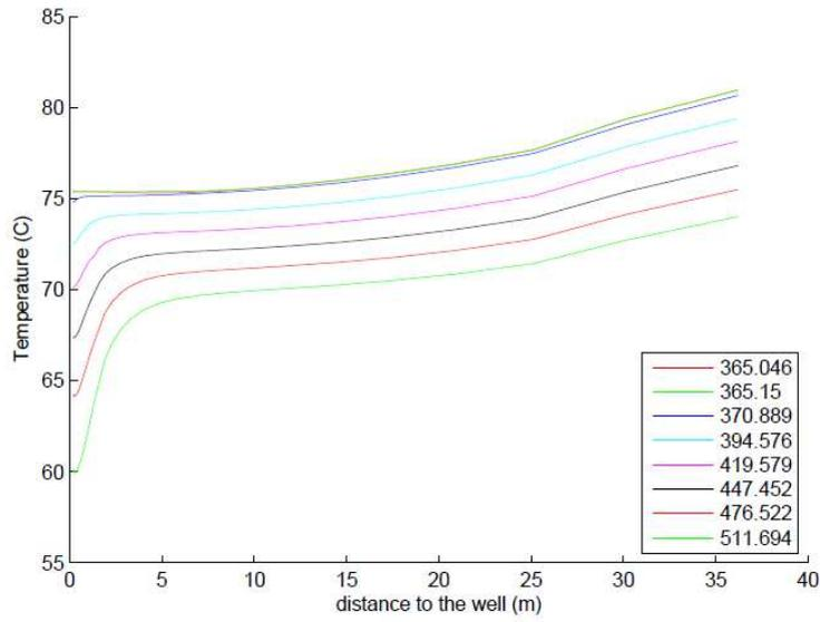
Figure 18. Initial temperature development in the fracture in the caprock. One line per time step (legend shows the time in days).
