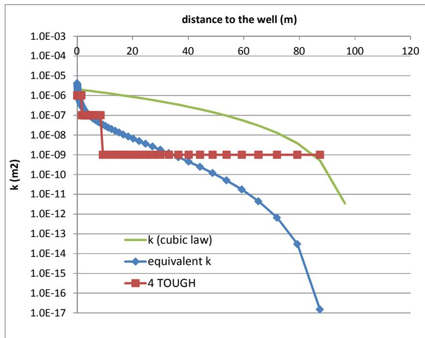
Figure 4. Example of permeability (k) as calculated for a 100 m long fracture with a maximum width of 5 mm showing k based on the fracture width (green line), the equivalent k corrected for grid block width (blue line) and k as entered in TOUGH2 (red line with squares).
