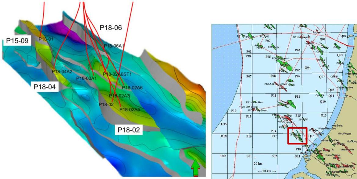
Figure 1. 3D view of the top of the P18 fields. Faults are shown in grey, well traces are shown in red. Reproduced with permission from (Arts et al, 2012)
