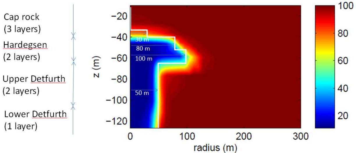
Figure 17. Temperature (°C) after 1 year and the extent of the fracture that is implemented in the reservoir model.
