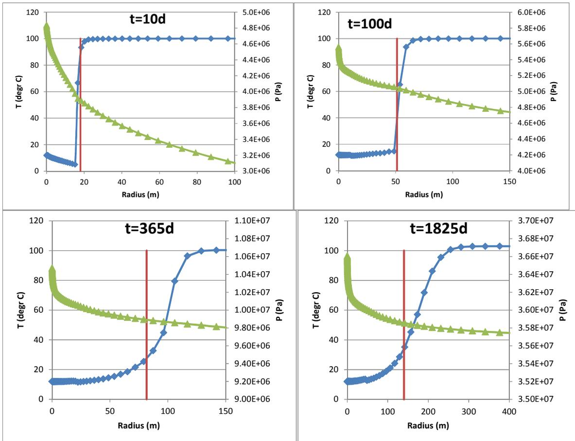
Figure 8. Temperature and pressure profile with distance from the well for four time steps: 10d, 100d, 1 year and 5 years. The red line indicates the extend of the fracture
