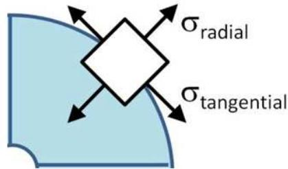
Figure 6. Representation of the radial and tangential component of the thermal stresses.
