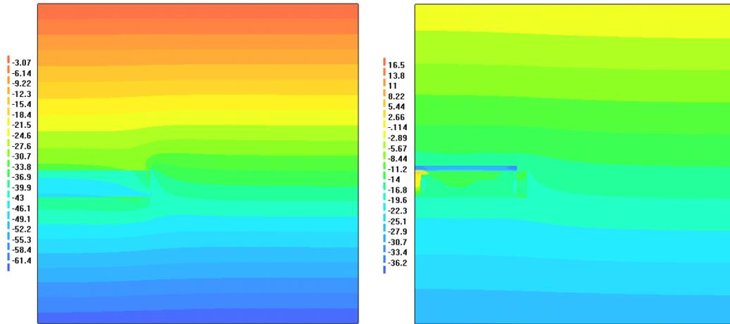
Figure 15. Test case, from left to right: state of stress (MPa) at the beginning of the injection (depleted reservoir) and after 1 year of injection.
