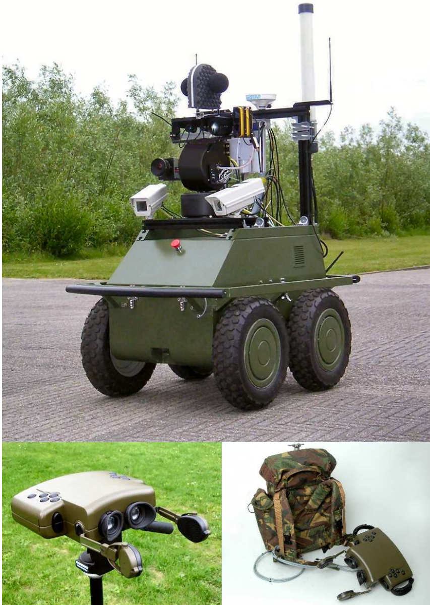
Figure 1.2: The top image shows the EyeRobot mobile robot demonstrator for reconnaissance and surveillance tasks. The two white cameras on the front are a stereo pair that is used for obstacle detection. In between these cameras is a pan-and-tilt unit that houses several cameras and microphones for observation functions. At the bottom, two images are shown of the Tele-Presence Binoculars.
