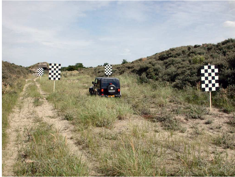
Figure 2.9: The test track in rough terrain used for our experiments. The test vehicle is driven over a straight path between the landmarks.
