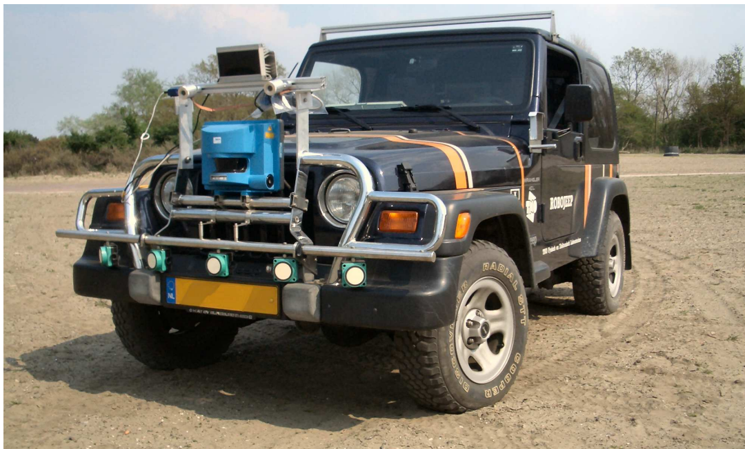
Figure 1.1: The RoboJeep robot vehicle developed by TNO. The top image shows a side view, where the DGPS unit is visible on the roof. In the bottom image, the front is visible with the LIDAR sensor and the stereo camera mounted on the bull bar.
