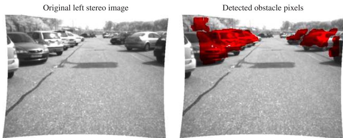
Figure 4.1: On the left, the original left stereo image is displayed. Detected obstacle pixels by the V-disparity technique are coloured red in the image on the right.
