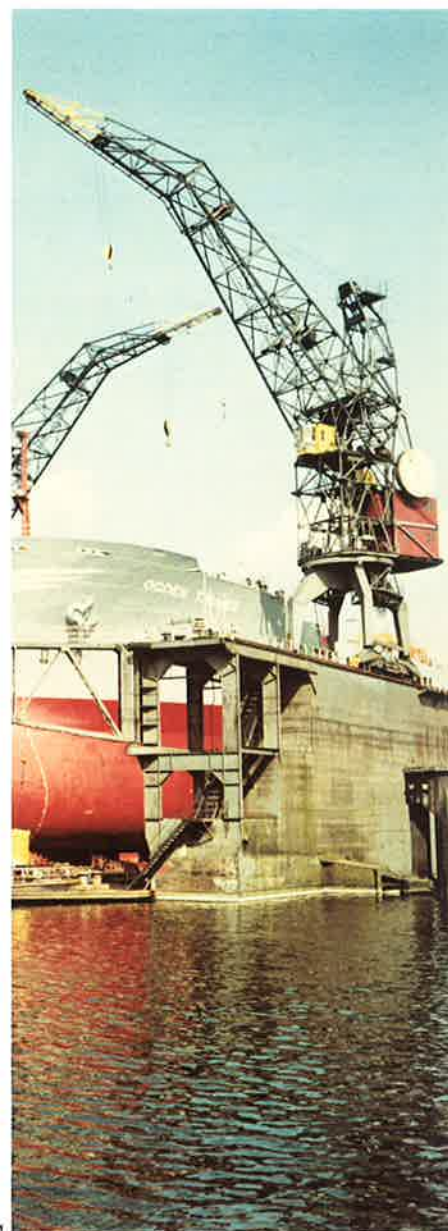
10. Base Unit for Mobil Oil. Total mass 957 tons, measured with 7 load cells each of them having a nominal range of 2500 kN.
